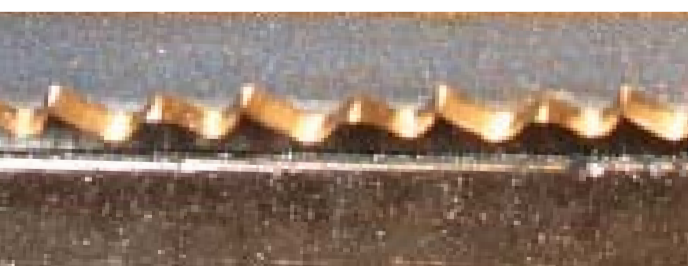
Crosscut tooth geometry. Jointing crosscut saw teeth creates triangular flats at the point of each tooth. These reflect light and help guide the sharpening process.
