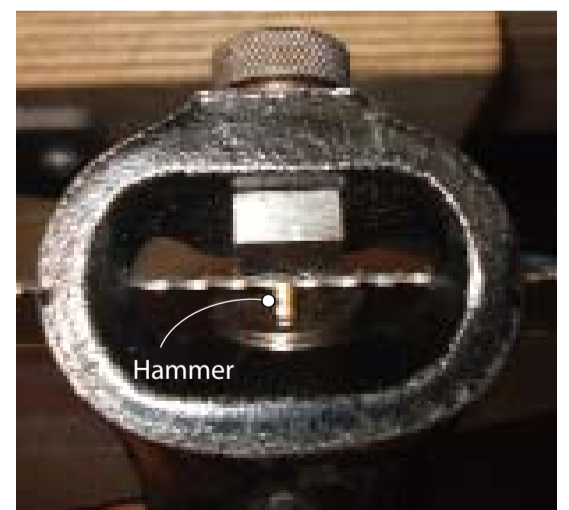
Set. Slip the saw set over the saw blade, rest it firmly on the toothline, align the hammer with a sawtooth, then squeeze.
