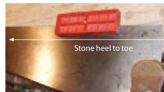
Stoning. To remove burrs left by the filing, and to remove set, make no more than four passes down each side of the teeth with a fine India stone or #600-grit diamond stone.
