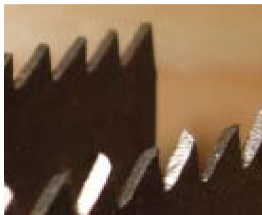
Rip teeth vs. crosscut teeth. Rip teeth (left) are shaped like tiny chisels and are shaped and sharpened by filing square across the blade. Crosscut teeth are shaped more like knives and are formed by filing at an angle to the blade.
