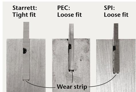
The more accurate the fit of the blade into the body, the less chance of a loose fit affecting accuracy and operation. A narrower wear strip will likely wear faster, changing the accuracy of the square in a shorter period of time.
