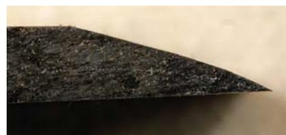
***Look closely.** The secondary bevel on this chisel is difficult to see in this picture. Part of the reason for that is that honing freehand rounds the bevel slightly. This isn't a problem as long as the angle at the very tip doesn't get too high.*
