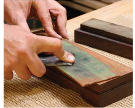
**Polish.** Fine scratches can be polished away using a leather strop charged with a polishing compound such as this chromium oxide.
