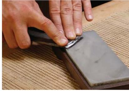
**Hone.** I use my finest stone to remove the wire edge created by my coarser stones. No reason to scratch the back on a coarse stone. I just work the area adjacent to the edge. I prefer to hone front to back so I use the corners of the stone.
