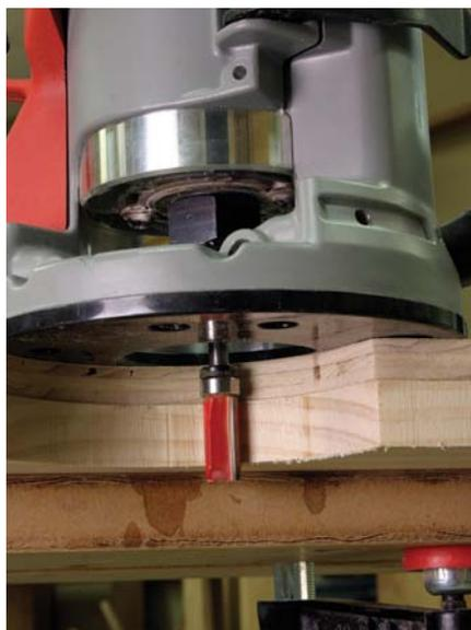
**Ready to rout.** Grab your router and before you plug it in, install a ½" straight bit, then adjust the depth of cut so that the blade hits your workpiece and the bearing rides on your pattern.
