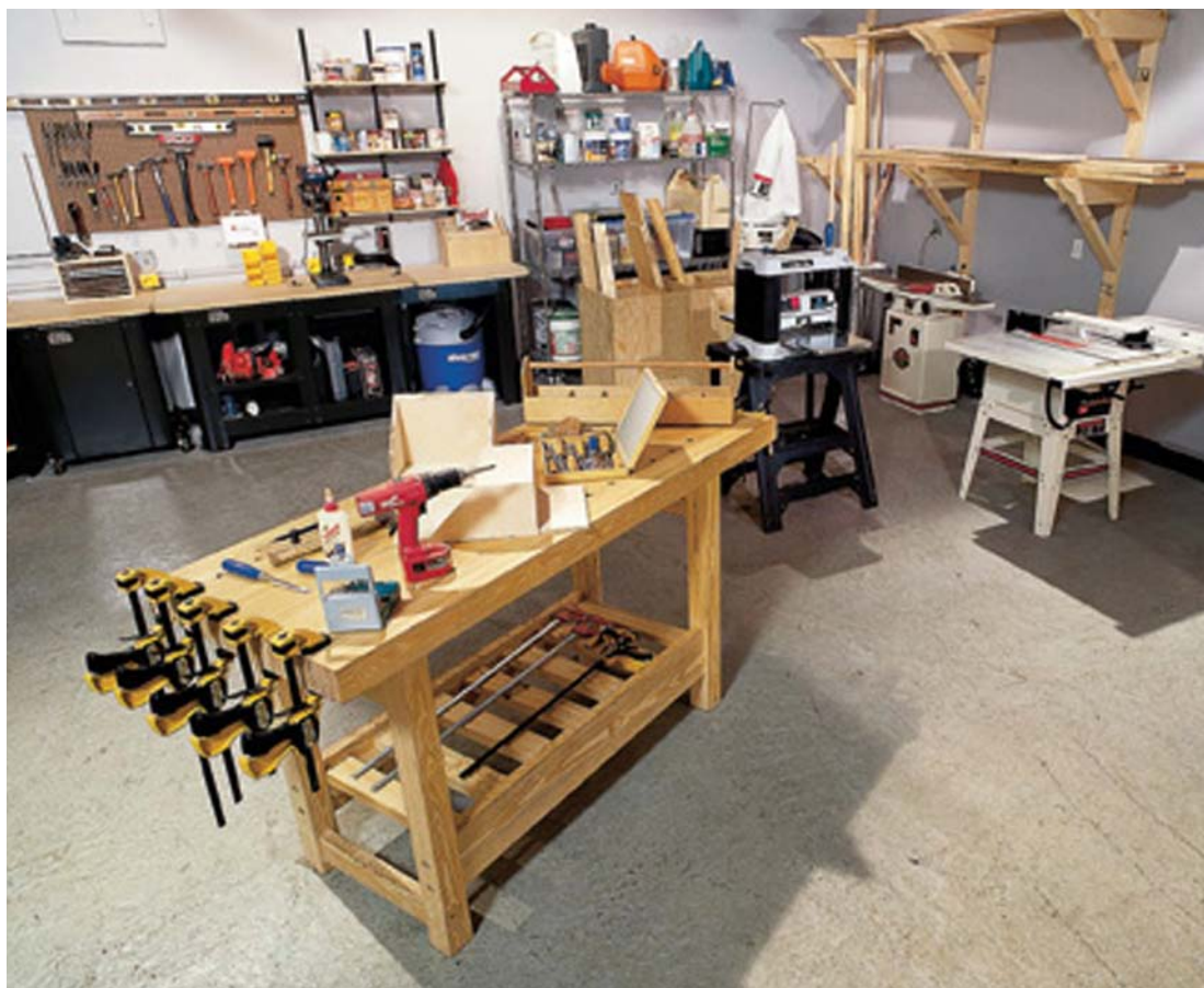
A good workbench is one item you should build into your plans from the start. We've put the bench in this shop so it's central to all the activity. It's just a short step away from the saw and planer, and only a few feet away from all the hand tools and other benchtop tools. And with it isolated in the center of the room, all four sides of the workbench can be used. You can order complete plans for this bench (which costs just $175 to build) from our web site at www.popularwoodworking.com . The plans are $9.95.
