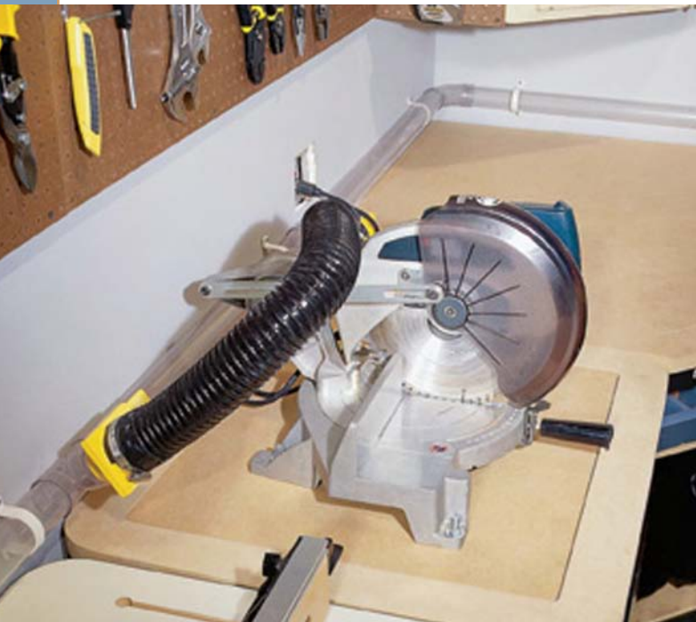
Here's a little closer look at the interchangeable drop-in panels and dust-collection hook-ups for the benchtop tools.
