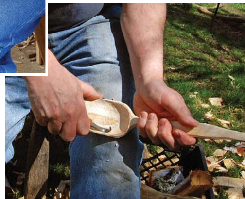
Across the bowl. A hooked knife gives you precise control as you shape the bowl.
