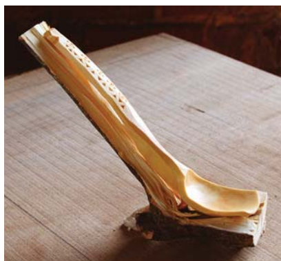
Crooked blank. From a crook comes a thin but strong spoon.
