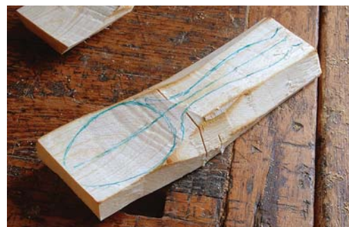
Pencil it in. After sketching the outline of the spoon on top of the blank, make relief cuts with a saw or hatchet to where the bowl meets the handle.
