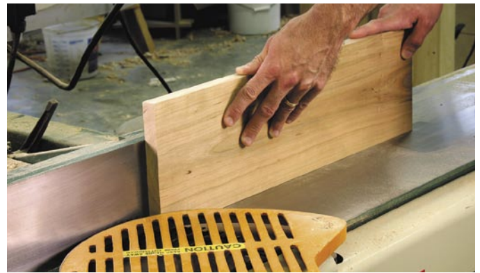
With the faces surfaced and parallel, a stop at the jointer ensures a 90° edge in relation to those faces – even if you cleaned that edge at the beginning.
