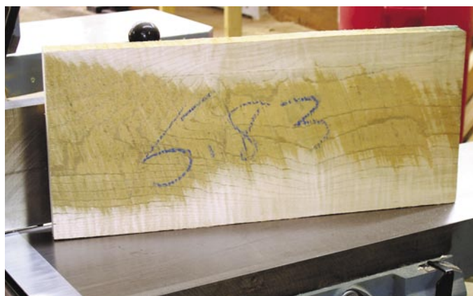
Flattening stock at the jointer does not mean to completely surface the face. This piece will sit flat and stable when it is sent to the planer.
