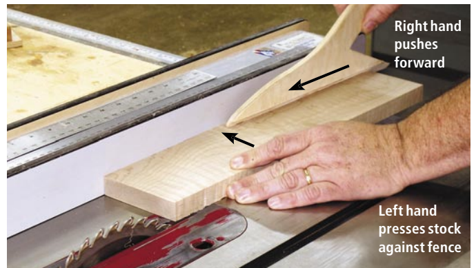
Push sticks can help guide your stock as well as hold it tight to the fence and table. They are invaluable tools in your shop.
