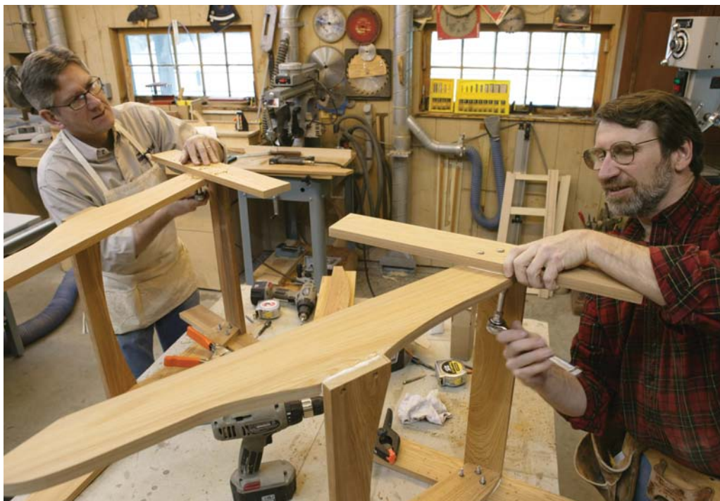
Bolt the legs and side members together, bolt head to the outside with a nut and flat washer inside. Seat the square shank below the head with a hammer blow. The shank will prevent the bolt from turning in the hole.
