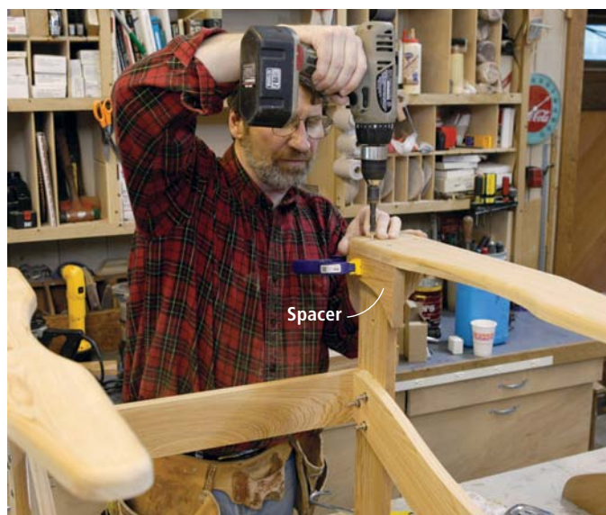
Use three screws to attach the arm to the leg and arm bracket. Carefully position the arm for a ¾" overhang of the leg. Use a spacer to help position it. The arm overhangs the front edge of the leg 1⅛".
