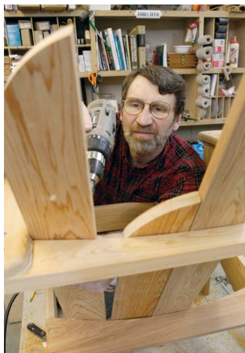
Start installing the back slats with the center slat first, then the outer slats. The last two intermediate slats are then easily positioned with equal spacing between their neighbors.
