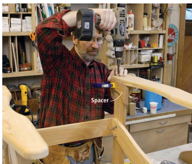
Use three screws to attach the arm to the leg and arm bracket. Carefully position the arm for a 3/4" overhang of the leg. Use a spacer to help position it. The arm overhangs the front edge of the leg 1 1/8".
