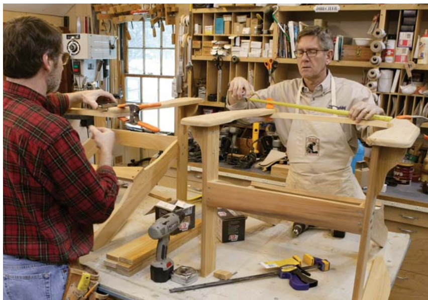
Hold the upper back crosspiece in place with clamps so that the arms are 20½" apart, then drill each side for two carriage bolts.
