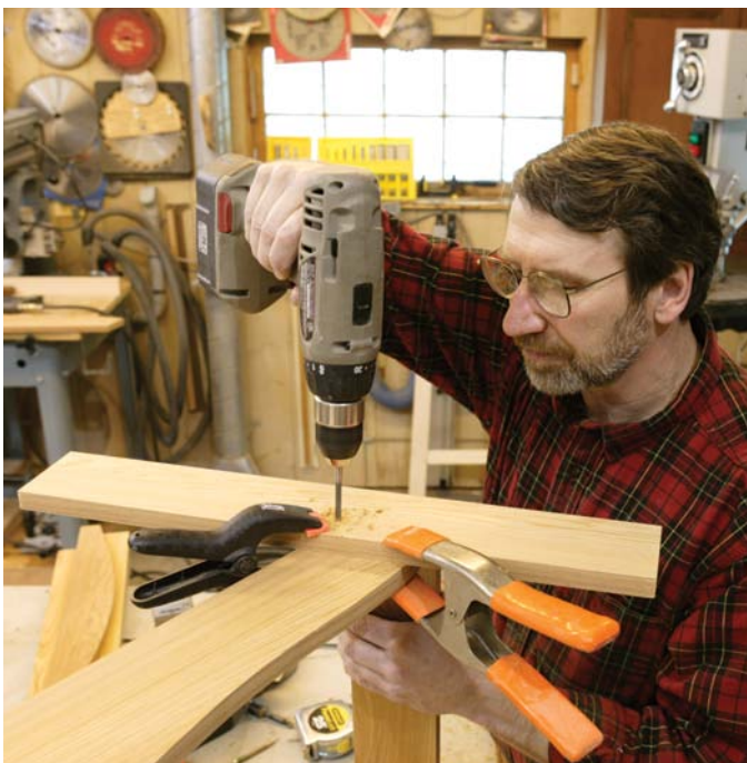
Arm installation over leg & bracket
