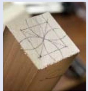
**Smaller octagon.** For the small octagon at the foot, mark the square you want to turn into an octagon, reset your compass and repeat the process.
