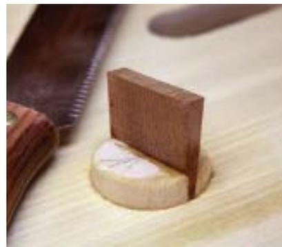
**Set for life?** Wedging the tenons will keep them tight even after the glue fails. To prevent splitting, the kerf in the tenon is perpendicular to the grain of the seat.
