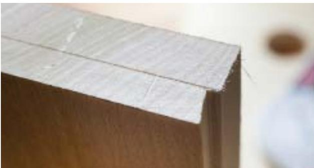
**Little triangles; big strength.** Here's the little triangular section that creates the dovetail, which was cut with a shoulder plane. The waste in the corner can be removed using a saw or chisel.
