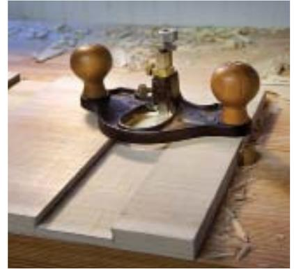
**Flat & finished.** Router planes excel at making housed joints perfectly flat. You could do this work with a chisel, but it would be a fussy process.
