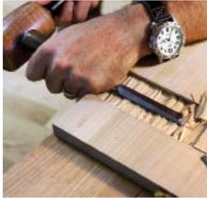
**Faster than you think.** A chisel can remove waste much faster than a router plane. Just keep an eye on the grain so it doesn't split below the final depth of the socket.
