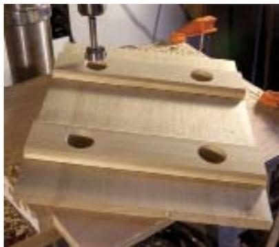
**Quick & flawless.** The platform raises the seat to the 16° resultant angle. The pencil lines ensure that the angle is in relation to the centerpoint of the seat.
