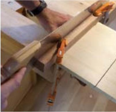
**Saw perfect walls.** The 16° guide is made from scrap and is clamped to the underside of the stool's top. An 8-point crosscut handsaw was used to make these four kerfs.
