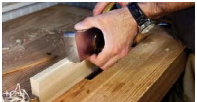
**Plane the middle.** There is so much friction in assembling a sliding dovetail that it's best to hollow out the middle of the joint with a few "stopped shavings" along the joint's bevel.
