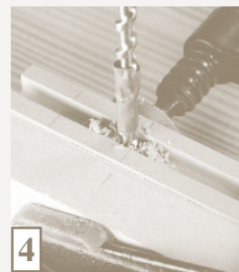
4 Generally, I mark only the auger bit with tape. The hole limits the depth of cut made with my chisel. Attempts to mark the depth of cut on the chisel are always a struggle.
