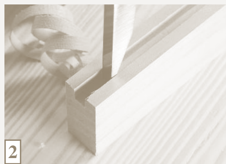
2 Here you can see the advantage of tool slaving. My chisel drops into the groove. The walls will guide the chisel.
