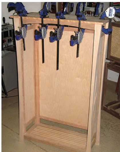
No nails needed. The frame of the top is glued to the front and back panels while the top's panel is doweled to the cabinet sides. Get your clamps ready.
