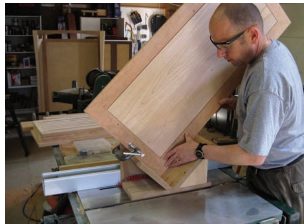
Jig it up. Splines reinforce the mitered corners on the top unit. To cut the slots, it's best to make a jig that slips over your table saw fence as it holds your assembly at a 45^\circ angle.
