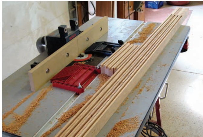
Identical curves. Use the shaped leg, along with a router and pattern bit, to create the remaining legs.
