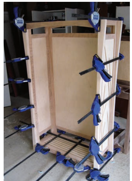
The case comes together. To fit the side panels between the front and back assemblies is not a challenge. But throw the case bottom into the mix and the balancing act begins.
