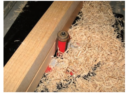
Identical curves. Use the shaped leg, along with a router and pattern bit, to create the remaining legs.
