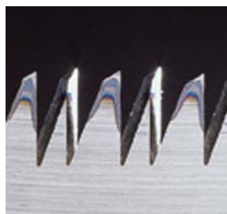
Japanese Crosscut Teeth • Note the long slender teeth and three bevels filed on each tooth. The tips are discolored from impulse-hardening.
