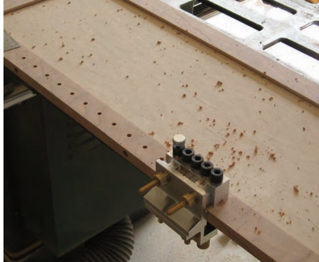
Scads of adjustment. A dowelling jig makes easy work of the many holes that need to be drilled for the adjustable shelves – or you could use a piece of pegboard. Whichever you select, make sure the holes are equally spaced so your shelves lie flat.
