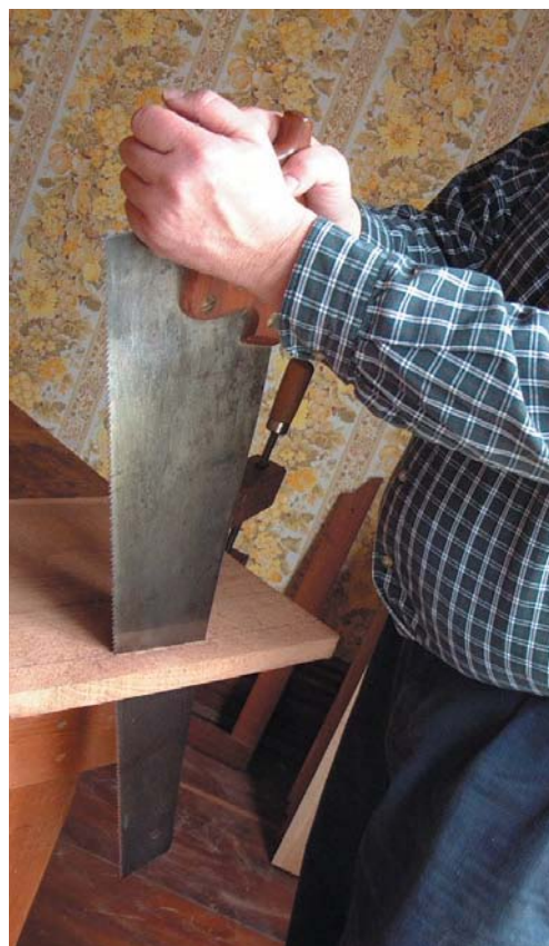
The Western handsaw, shown here being used by Don McConnell with an overhand rip grip, cuts on the push stroke.
