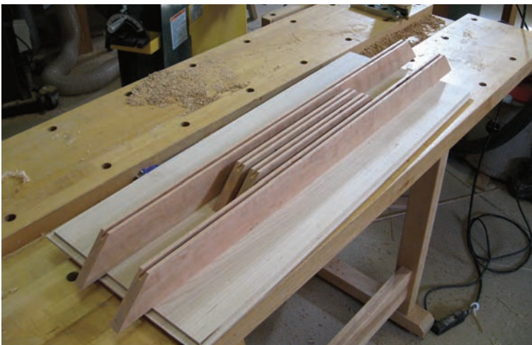
Keep them centered. The key to a perfect fit is to keep the grooves in the middle of the top's frame pieces, and to work with straight, flat material.
