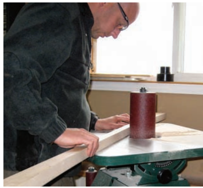
Shape a gentle curve. Use a spindle sander to shape one leg exactly to your layout line.
