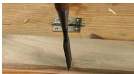
Use a chisel define the sides of your mortise. Then, chop a series of shallow cuts in the waste area of the mortise, which will make the waste easier to remove.
