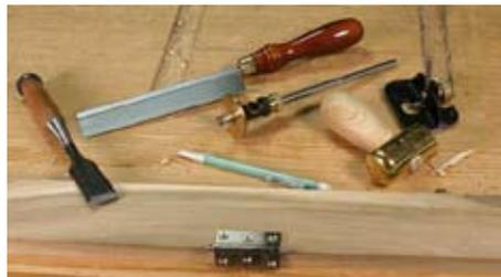
From left: A 1" chisel, a gent's saw, a cutting gauge, a Glen-Drake #4 Tite-Hammer and a Veritas small router plane (and a mechanical pencil).
