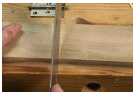
Use a gent's saw or other small saw to make a series of shallow cuts in the waste area of the mortise. Define the mortise sides with a chisel.
