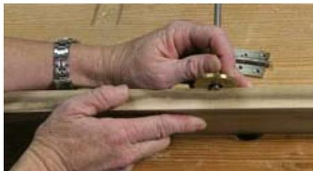
Scribe a line along the edge to define the bottom of the mortise. If you don't have a cutting gauge, use a pencil to mark the bottom edge, or scribe a line with marking knife or X-Acto knife.
