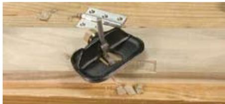
If you have a router plane, set the cutter depth to the bottom of your mortise and remove the remaining waste.
