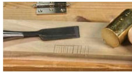
Use your chisel (bevel-side up) to define a shallow trough along the back edge of the waste area. (This will help to avoid blowout when removing the waste, especially if the back of the mortise is near the edge of your workpiece.)
