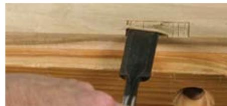
Chisel out most of the waste. You may want to repeat Step 5 a few times to help ease waste removal. If you don't have a router plane, continue to remove the waste with your chisel until you've defined the flat bottom of the mortise.
