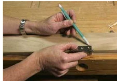
Hold your hinge firmly in place on the workpiece and mark a line at the back edge and side edges. Better yet, scribe the lines with a marking knife.
