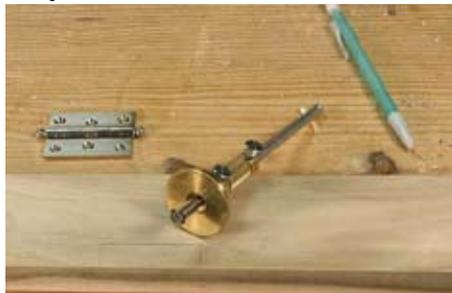
Reset your cutting gauge to define the line at the back edge of the mortise (if you scribed the line with a knife instead of marking with a pencil, this step is unnecessary).
