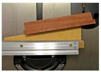
**9** Here is an overhead view prior to cutting the second slope. Note that the two slopes will converge at the bottom of the marker.
