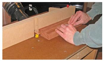
1 Cut the large rabbet in small increments at the router table. Alternatively, hog out most of the waste on the table saw. The wood must be free of internal stress.
