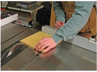
6 After setting the miter gauge at the dovetail angle, crosscut to make the wedge.
