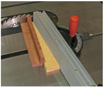
This shows the wedge and workpiece setup in crosscutting the first slope of the marker. Sandpaper on the front of the wedge will prevent sliding of the workpiece (which would result in inaccurate surfaces on the marker)
