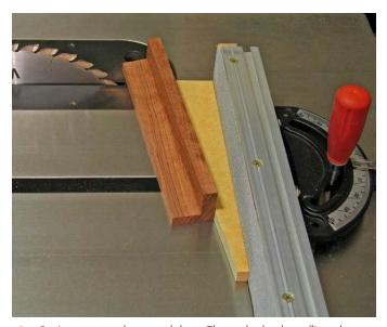
8 Setting up to cut the second slope. The wedge has been flipped. The workpiece, with the first slope cut, is extended past the blade to produce a marker about  $1^1/4^{\prime\prime}$  wide.
