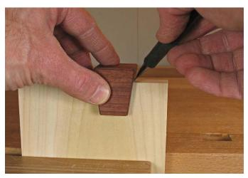
10 The finished marker in use. It has enough width to register firmly on the end of the board, but is not so wide as to be unstable when working near the edge of a board with some of the marker overhanging. These markers work for tails-first or pins-first dovetailing.
