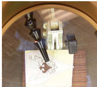
Reverse direction. To cut out the inlay, feed the piece to the saw blade in the opposite direction.
