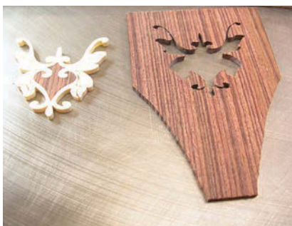
Interior fit. Place the interior piece(s) in the inlay
