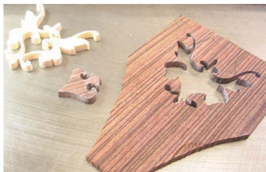
Get ready. Divide the components to prepare for the final assembly of the inlay.
