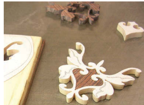
Waste extraction. Here's the inlay piece completely cut out. The separate pieces at the top are waste.
