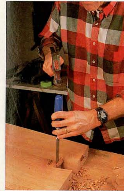
After sawing out the bulk of the waste with a coping saw, chisel the remaining waste. Make certain your cuts are perpendicular to the face. After cutting halfway down, turn the panel over and work from the other side to avoid tear out.
