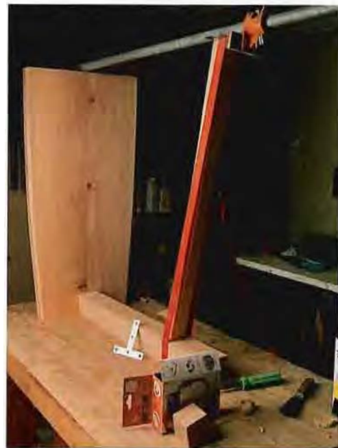
To clamp the tapered leg in place, use a band clamp. The pipe clamp is essentially used to maintain the leg in the right position. The "T" bracket is later screwed to the top of the leg and is used to secure the leg to the underside of the top.
