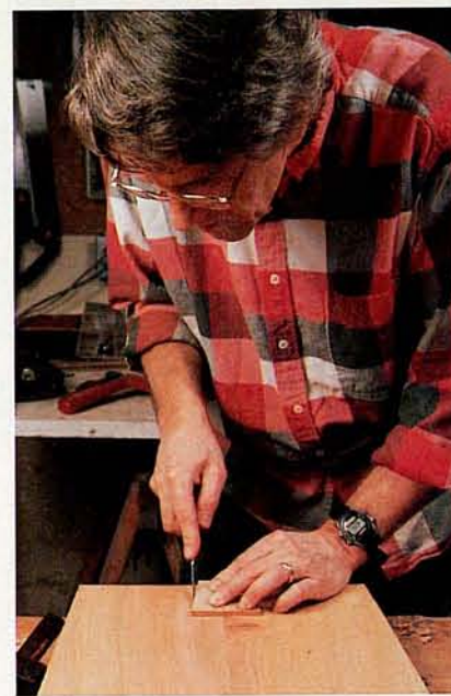
Mark the outline of the dovetail to be cut in the center of the bottom edge of the panel end using a trim piece of the actual beam. With the dovetail shape already cut on the beam, an accurate layout is assured.
