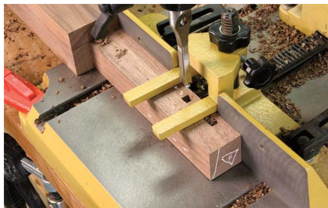
Make your mortises a little deeper than the tenons are long. The two mortises in the legs may end up meeting a bit at one corner, but that's OK. You're not removing material that will ultimately assist in strengthening this joint.
