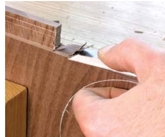
A wide paring chisel makes short work of the waste left from cutting the edge shoulders. Work carefully here and avoid cutting past the shoulder line. If you are skittish, use a 3/8"-wide chisel, which will keep you clear of the shoulders, but it will be a bit harder to steer in the cut.
