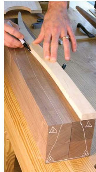
Marking walnut is a challenge. After trying a variety of pens, the best was a white ink pen available from an art supply store. The Sakura Pen-touch (gellyroll.com), costs about $2.50. Here's a tip about its tip: A light touch will give you a fine line.
