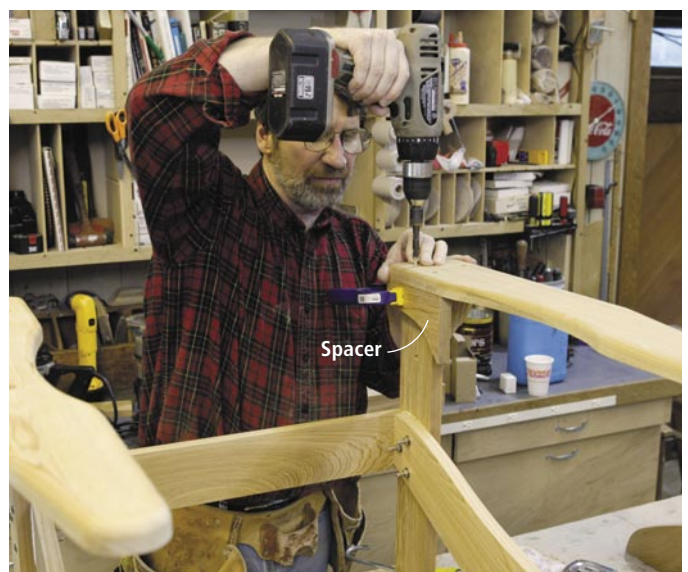
Use three screws to attach the arm to the leg and arm bracket. Carefully position the arm for a \frac{3}{4} " overhang of the leg. Use a spacer to help position it. The arm overhangs the front edge of the leg 1\frac{1}{8} ".
