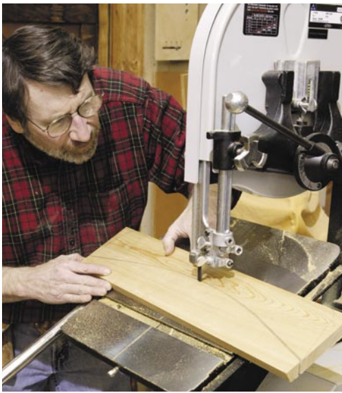
Cut the upper rear crosspiece's inside curved edge at a 30° angle. Then return the band saw table to 0°, or square, and cut the round ends.
