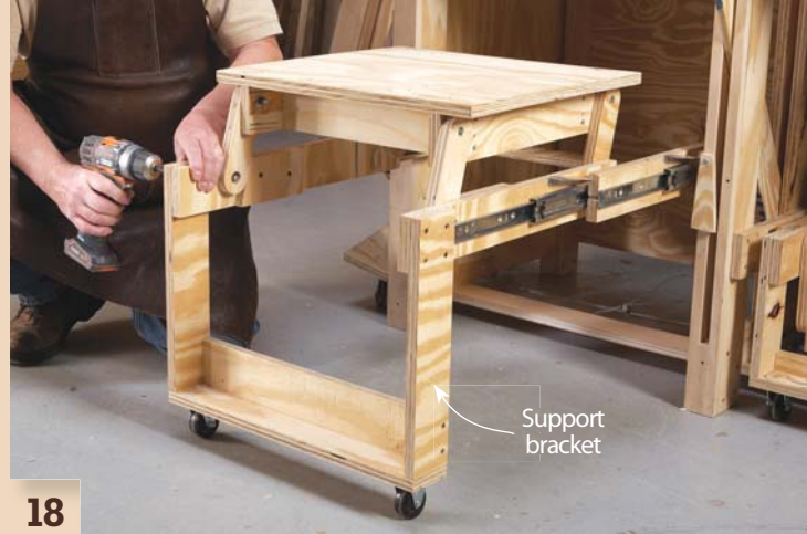
18 Install the support bracket to complete the tool platform.
