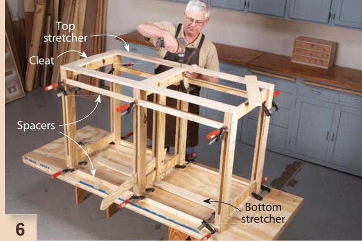
6 Assemble the bench cabinet by attaching stretchers and cleats after installing spacers to properly position the frames. Attach the back to complete the job.
