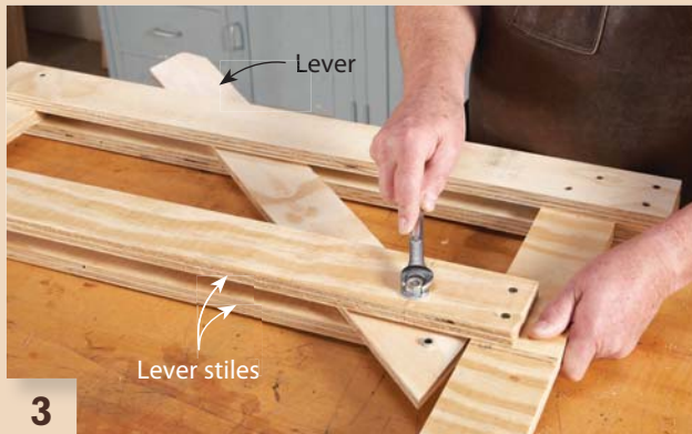
3 Install the lever in the middle frame after attaching the lever stiles. The lever raises the bench onto its casters by means of a cable and pulleys.
