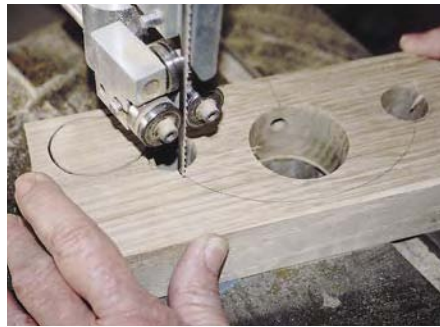
The plane body is sawn on the band saw.
