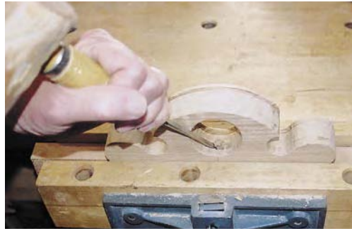
Carve the recess for the head of the thumbscrew as shown here.
