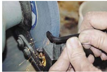
Grind the cutter to a 30^\circ angle. Grinding manufacturers don't recommend side grinding but I've always felt safe.
