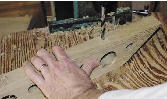
Drill the \frac{3}{8} " hole for the thumbscrew. The larger 1"-diameter and 2"-diameter holes can be either drilled or sawn depending on your woodshop's drilling capabilities.
