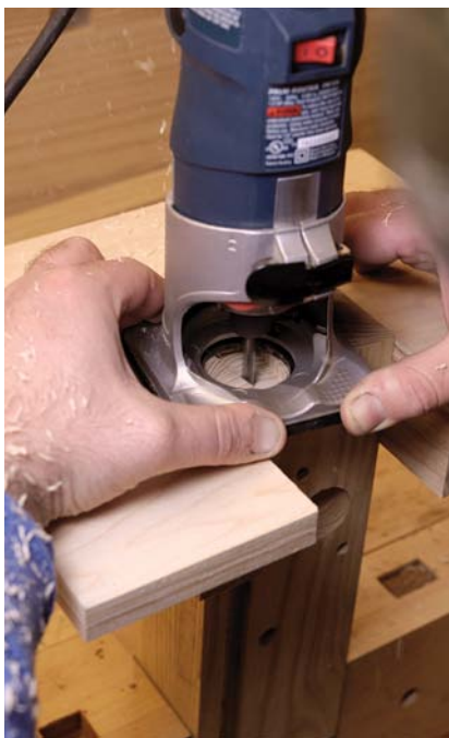
Route the waste. A trim router with a \frac{1}{4} " upcut spiral bit gets rid of most of the initial waste.
