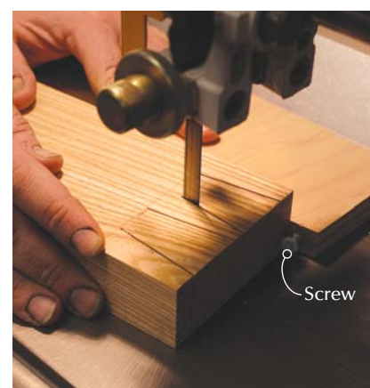
Opposing angle. After changing the screw stop, cut the opposing angle, flip and repeat.
