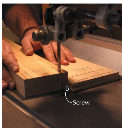
Tandem slide. Slide both the spacer and workpiece along the fence to make the cut.
