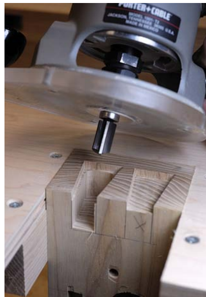
First pass. Get rid of most the waste on your first pass.
