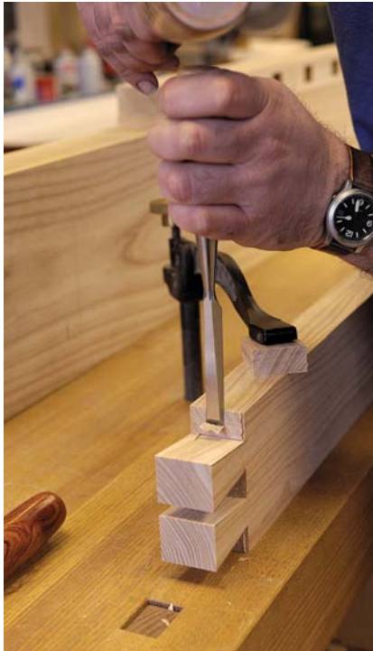
Chop by hand. Chiseling the end grain allows controlled precision.
