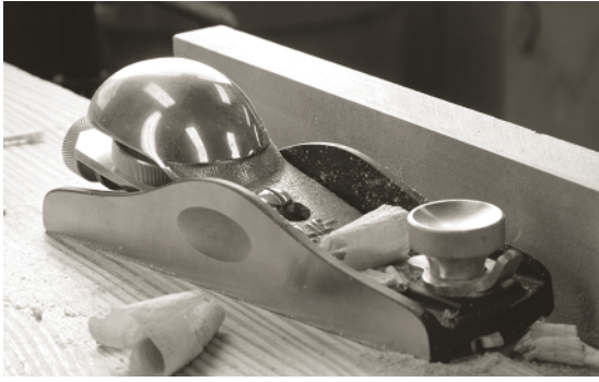
A BLOCK PLANE CAN SKIM the machining marks from the edges of your boards, leaving a ready-to-finish surface behind.
