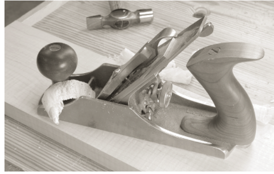
THE SMOOTHING PLANE IS THE thoroughbred of the shop and is kept highly tuned. Make sure the shavings come out of the center of the mouth.
