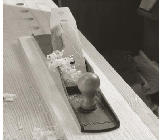
THE JOINTER PLANE EXCELS AT truing stock , both the long edges and faces of boards. The pencil marks on the wood in the photo are low spots found by the plane after two passes over the board – which was fresh from the planer.
