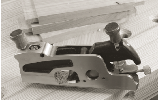
THE SHOULDER PLANE IS A joint-trimming maestro . This tool will fit tenons, rabbets, raised panels and shiplaps with ease.
