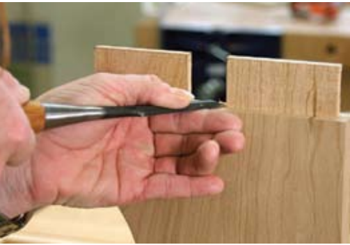
Split tenon. A 6½"-wide tenon is too big, so I split it using a coping saw then chiseled out the remainder of the waste.
