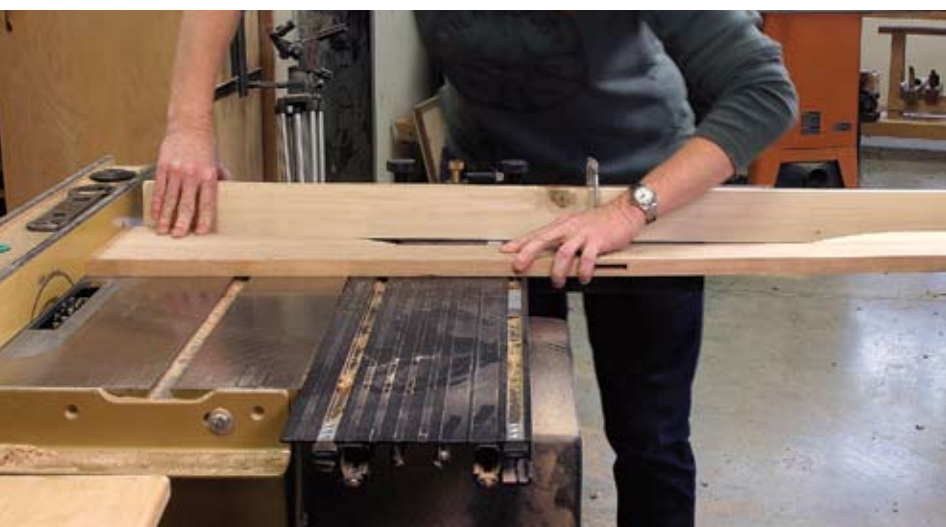
Jigged up. Because the feet created a non-flat surface, and the sliding table is shorter than my workpiece, I simply clamped a flat piece of scrap to the fence against which I could hold the rail while I made the tenons.
