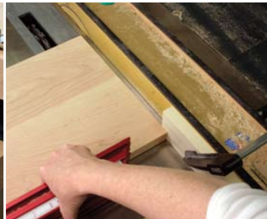
More jigs. Again faced with secure workholding problems at the table saw, I used a handscrew attached to the sliding table to support one end, and a stepoff block at the other to safely locate the groove for the bottom fixed shelf.
