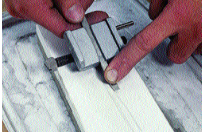
When honing narrow chisels, this is the best way I've found to keep things steady and square. Put one finger on the cutting edge; put the other behind the jig to move it.
