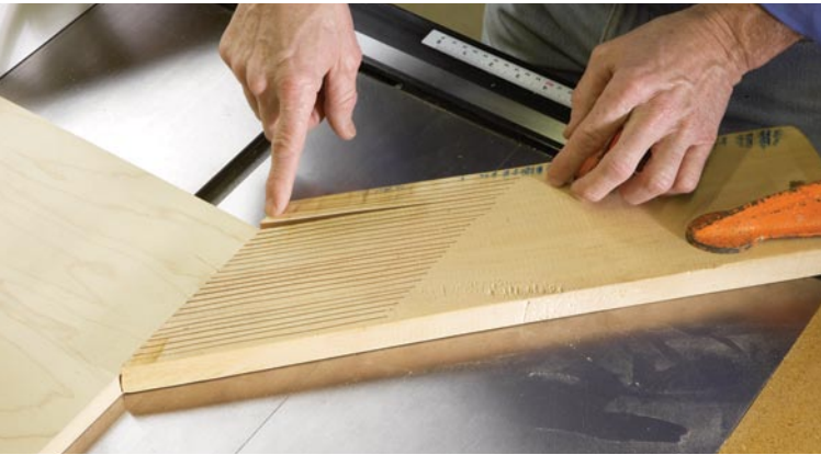
A proper featherboard. The fingers of a featherboard are consistent in size and springy, as shown. You can clamp them to the table or to the fence to help improve the safety of many operations.
