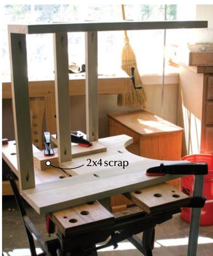
**Quick and easy screwing jig.** A scrap of 2x4 is clamped to the Workmate to serve as a guide and support for screwing the step supports and back brace in place on the side panels.
