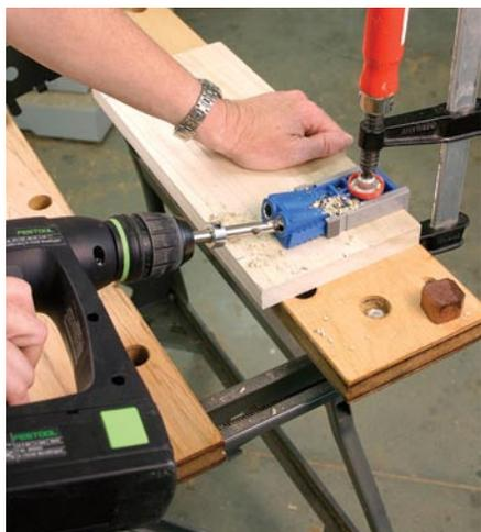
**Shaker-inspired step stool.** Don't let the panel glue-up scare you. This step stool (useful in just about any room of the house) is easy to build, using pocket screws as clamps and to add strength.
