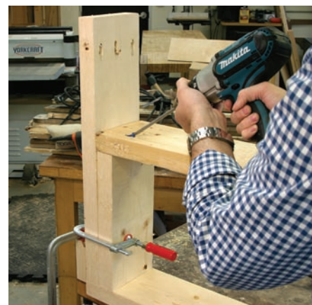
Scraps for a shelf. Use two 10¼" scraps to keep your brace centered and level.
