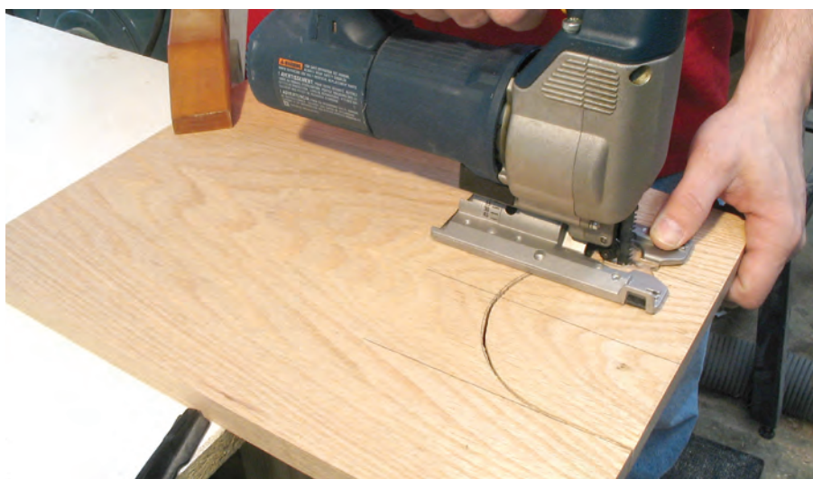
After marking the 5"-diameter circle and extending the marks down to the bottom of the legs, use your jigsaw to cut out the arches on both legs. Take your time in the curve. It's easy to cut outside your line.
