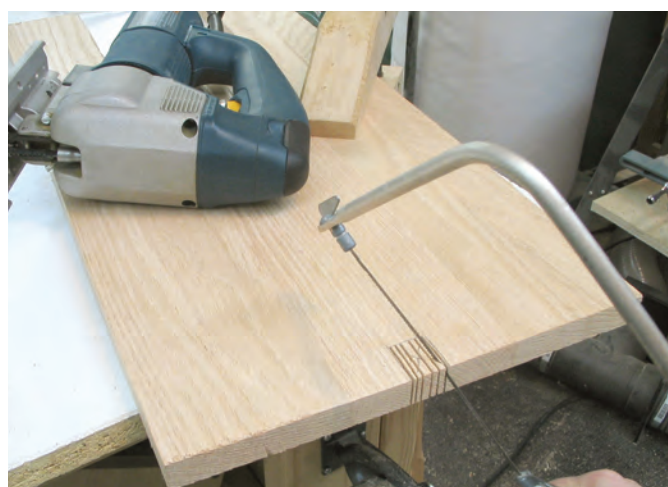
After marking the 5"-diameter circle and extending the marks down to the bottom of the legs, use your jigsaw to cut out the arches on both legs. Take your time in the curve. It's easy to cut outside your line.
