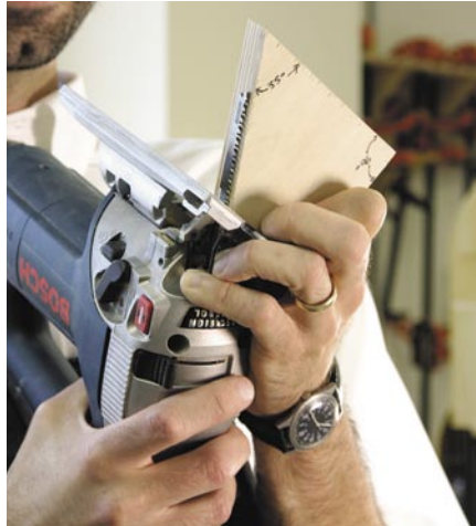
This scrap of wood acts as a reliable way to set your jigsaw's base to 35°. I found a protractor difficult to balance on the base and not nearly as accurate.
