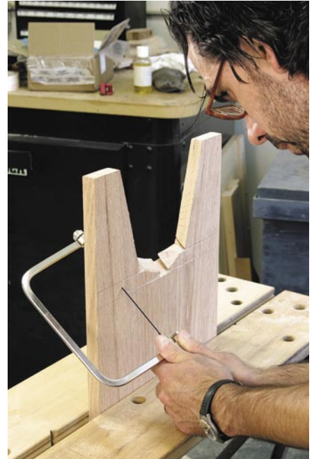
You can rotate the blade in its frame with a coping saw to make a tricky cut like this very easy.
