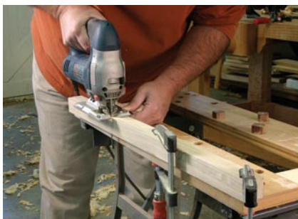
Cut with a jigsaw. If you begin the taper cut at the foot, the task gets easier as you move up the leg. Just make sure to clamp the waste area off the side of your workbench.
