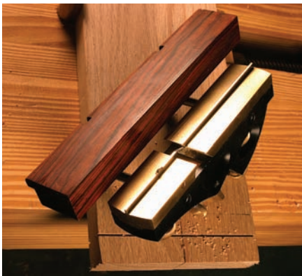
Innovative. The dado sole of the HP-6v2 has a remarkable slitter in front of the cutter that slices the cross-grain, eliminating chip-out.
