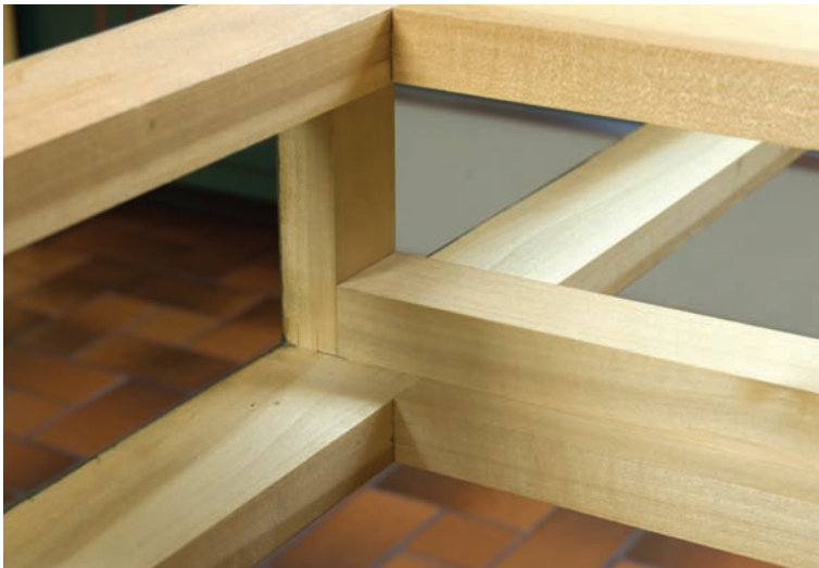
Sturdy framing supports multiple drawers in a table. A vertical divider mortised into upper and lower rails stiffens them. The runner and kicker, also mortised into the rails, double as cross members. The drawer guide is glued to the runner.
