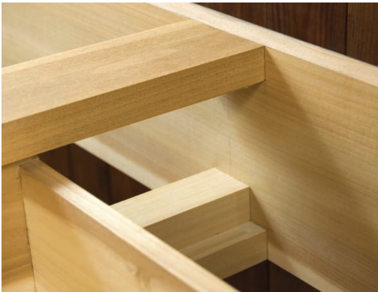
At the back, the runner and kicker are mortised into the apron.
