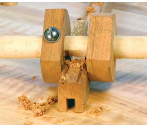
**Find the magic angle.** Start with the cutter at about a 45° angle and push or pull to produce a shaving. On curved work, you will need to reverse direction often to work with the grain.
