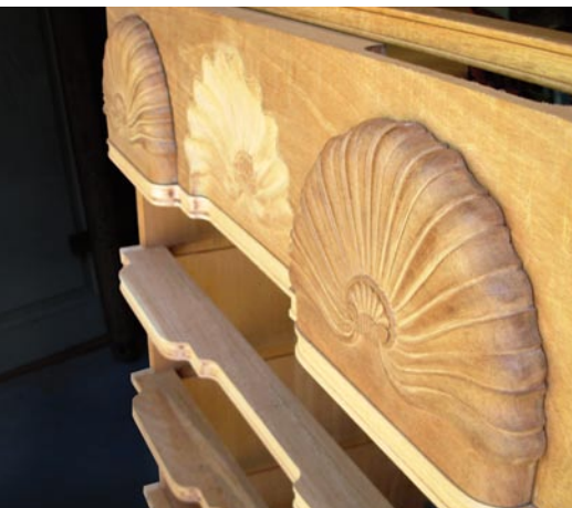
Quick profiles. Intricate detailed profiles can be cut quickly with a scratch stock, after the shape is formed.
