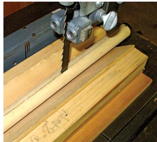
**Slot in the center.** A V-shaped fixture on the band-saw table holds the dowel in position to cut a slot down the middle.
