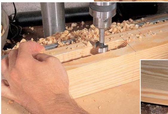
*After you cut your tenons, lay them directly on your work and use the edges like a ruler to mark where the mortise should start and end (top). Use a 1" Forstner bit in your drill press to cut overlapping holes to make your mortise (middle). Now square up the edges of the mortise using a mortise chisel and a small mallet (right).*
