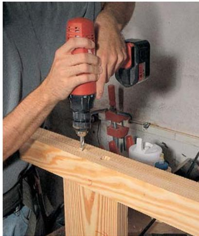
*Drilling the  $\frac{3}{8}$ " holes for the bolts is easier if you do it in this order. First drill the holes in the legs using your drill press. Now assemble the leg and front rail. Drill into the rail using the hole in the leg as a guide (left). Remove the leg from the rail and continue drilling the hole in the rail. The hole you drilled before will once more act as a guide. You still need to be careful and guide your drill straight and true (right).*
