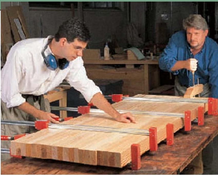
When you glue up your top, you want to make sure all the boards line up. Lay down your glue and then clamp up one end with the boards perfectly flush. Then get a friend to clamp a handscrew on the seam and twist until the boards are flush. Continue clamping up towards your friend, having your friend adjust the handscrews as needed after each clamp is cinched down.
