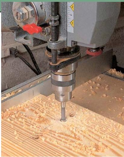
The mortises in the front rails are also made on the drill press. Make them  $1\frac{1}{4}$ " deep to make sure you can get a washer in there. If you can't, try clipping an edge off of the washer.
