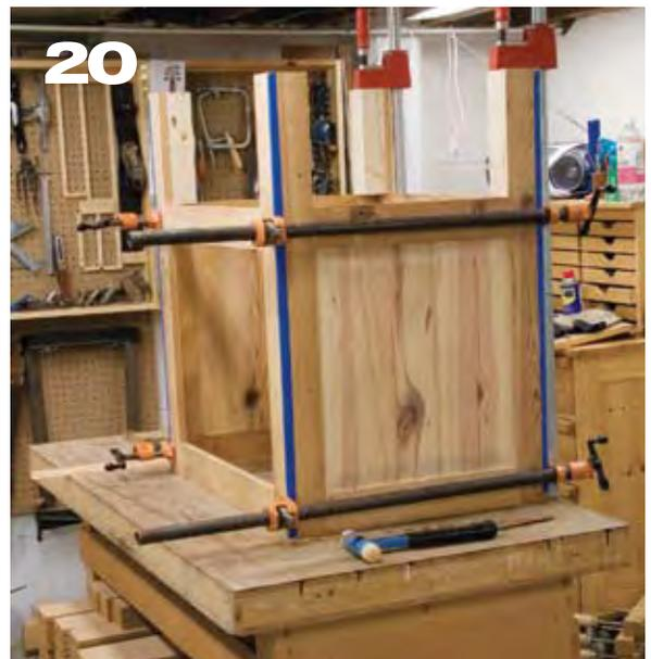
After the glue is dry, glue the front and back assemblies together. The cabinet is now assembled!
