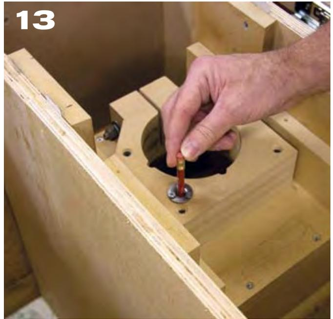
Drop a pencil (be sure it's long enough!) through the T-nuts and make a mark on the shelf of the inner box. Remove the carriage and drill a  $\frac{1}{2}$ "-diameter hole at this center-marked location. The threaded rod will protrude through this hole about 1".
