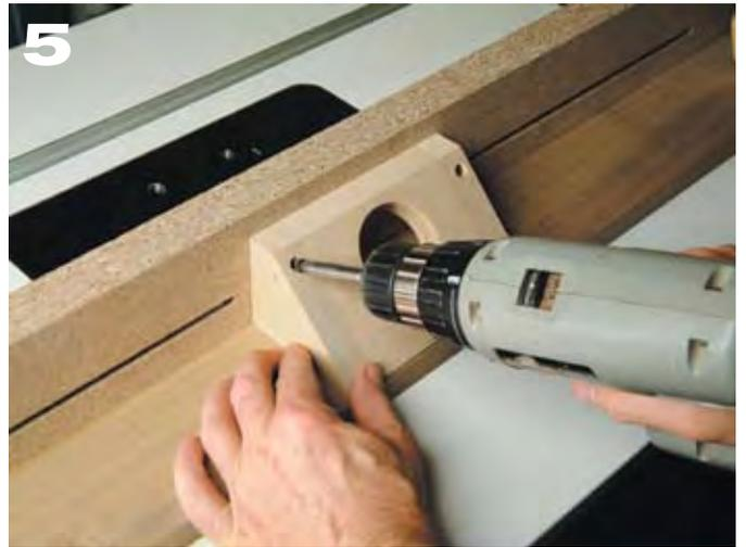
The dust hood for the fence is made from three pieces of MDF. Cut a hole in the hood to fit your dust collector or shop vacuum hose. The front piece is cut with a 45° bevel on both long edges. Cut a 45° angle to fit the end pieces to the front piece. You are now ready to start routing!
