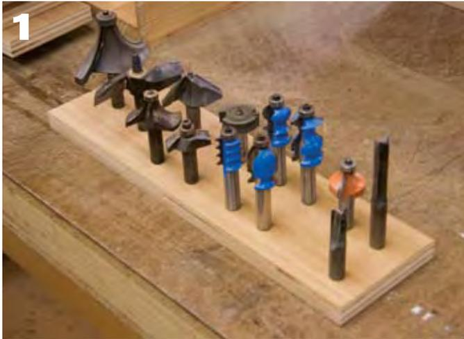
Cut out the pullout parts. Arrange your bits on the shelves. These are the largest cutter I have and they all fit on one shelf. I marked the hole locations and drilled them about halfway through the shelf.
