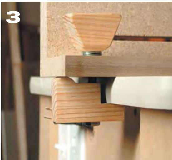
Because I'm cheap (or frugal), I make a lot of my fittings. The hold-down clamps are no exception. All you need are two bolts, two flat washers and two T-nuts. To install the T-nuts in the knob, drill a stopped-hole large enough to fit the entire nut. Then drill a through-hole just large enough to clear the nut's body. As the knob is turned, the T-nut pulls tightly against the bottom of the stopped hole.
