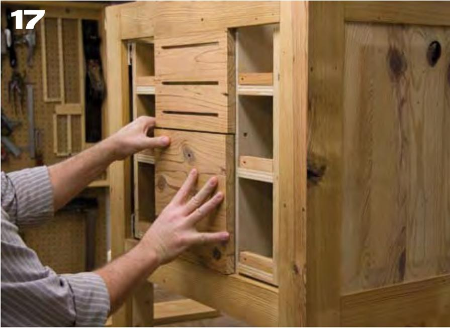
Use double-sided tape, applied to the front edges of the drawer sides and bottom, to hold the drawer front in place. Remove the drawer, glue the front to the front edge of the drawer bottom install screws through over-sized holes in the glue blacks.
