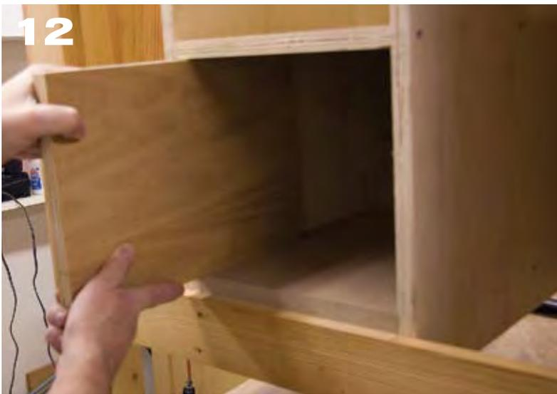
**12** Now, put the bottom in the opening and fit the sides to the space. Fit each side as there could be slight differences in the drawer opening. Finally, assemble the drawer. Attach the sides to the back, then center this assembly on the bottom. The sides should be about  $\frac{1}{8}$ " in from the side edges of the bottom.
