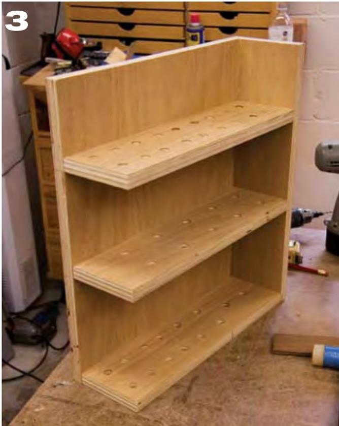
Screw the pullout parts together. I made the right-handed pullout for my router bits with  $\frac{1}{4}$ " shanks the left-handed pullout for my  $\frac{1}{2}$ " bits.
