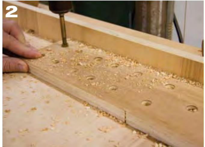
I drilled the rest of the shelves with two rows of holes spaced fairly evenly, just using my eye to gauge the distance between holes. I drilled three shelves with  $\frac{1}{2}$ " holes and the other three with  $\frac{1}{4}$ " holes. I ended up with ninety holes total – more than enough for now and the future.
