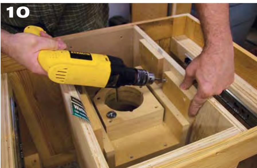
Now install the shorter dovetail keepers. The top bracket will be installed on the top of these keepers, so they are  $\frac{3}{4}$ " shorter than the other two keepers. Push the keepers snugly against the dovetailed guides, then install two screws. Note the spacers on the keeper on the left. The keepers need to be firmly against the body of the carriage, so some adjustments may be necessary.
