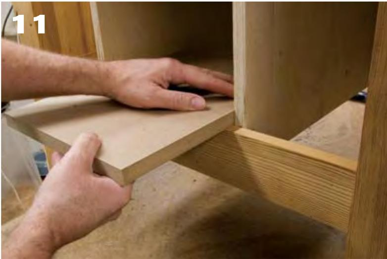
**11** Cut out the drawer parts. First, fit the drawer bottom into the drawer opening in the box. Trim as needed so the bottom slides smoothly in and out.
