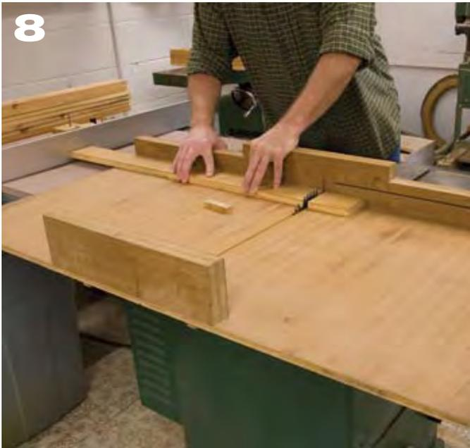
... then I slid this squared along the saw's fence (which has been set to the finished-length cut of the leg part) and made the final cut. This is a safe cut because the sled supports the leg part as it rides along the fence.
