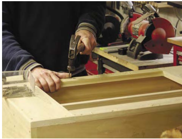
Carefully drive the nails that attach the face frame. (If you miss and ding up your stock, don't despair. Just spoon a bit of water onto the ding. As the fibers swell to accept the water, the surface of the wood will return to its original configuration.)
