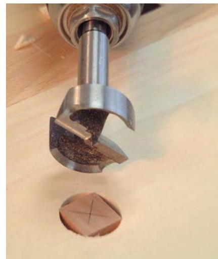
A smaller hole is easily made bigger by pounding a temporary plug in place before drilling the new hole.
