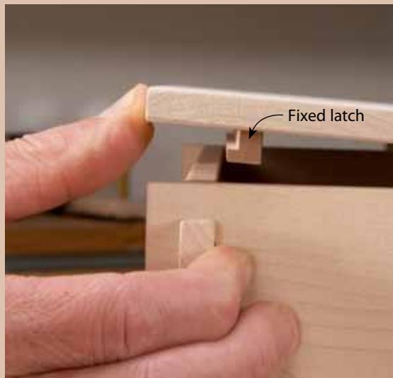
**Opening the box is a bit of a puzzler**, because the spring-latch system is completely hidden when the lid is closed. Here's how the system works: Tabs at the ends of the spring latch flex about 1/4" (above, left). These tabs fit about 3/16" into the latch groove in the back of the box. When the lid is pressed from the front (above, right), the spring latch flexes
