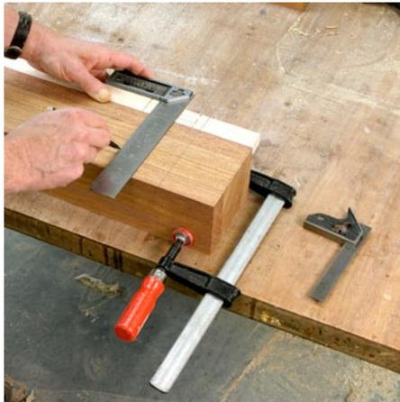
F-style sliding bar clamps are next on my list. I use the smallest ones (4" and 6") the most, usually for grouping parts together during layout, attaching jigs and hold-downs to the fence on the table saw or router table, and for holding parts and subassemblies to the bench. In these smaller sizes, the light-duty models are more than adequate, and at \$5-\$6 each,
