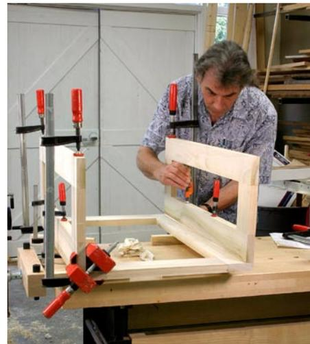
adjustments with the standard F-clamps with one hand by putting your thumb on the sliding part of the clamp at the bar and pushing or pulling. Stay with the basic ones – you don't even need the ones with the clutch plates; they will only slow you down.
