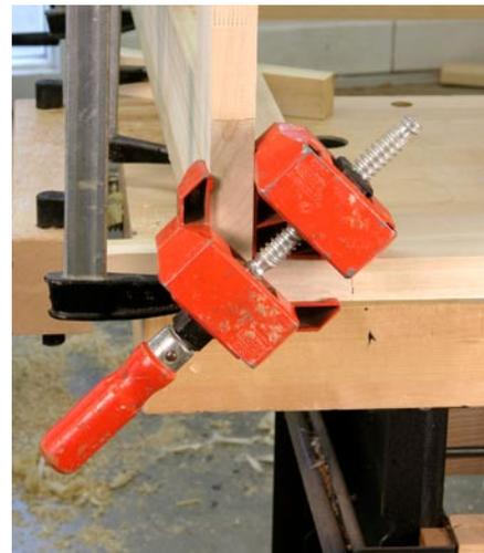
The problem is that as you apply pressure to the joint, the two parts tend to slide apart. Picture-framer's clamps will hold two mitered parts in place, but like the corner clamps, they don't pull the joint together. What you need is a way to squeeze the joint together, applying force
