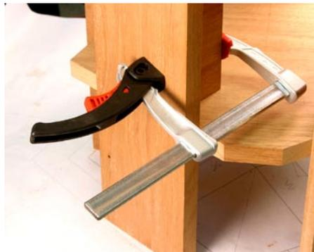
A new variation of the F-style clamp is shown in the middle picture below. Called a Kliklamp, this tightens with a ratcheting lever instead of the traditional threaded handle. It's quick to use and generates just the right amount of pressure. It's a welcome addition to our shop.
