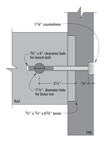
By far, the most popular way to bolt a bench together is to use a bed bolt system. You can, in fact, use bed bolts from a reproduction hardware company. Or you can use hex-head bolts from the home center. Use two bolts in each joint – eight bolts total per bench. Cheaper, yes. Classy, no.
