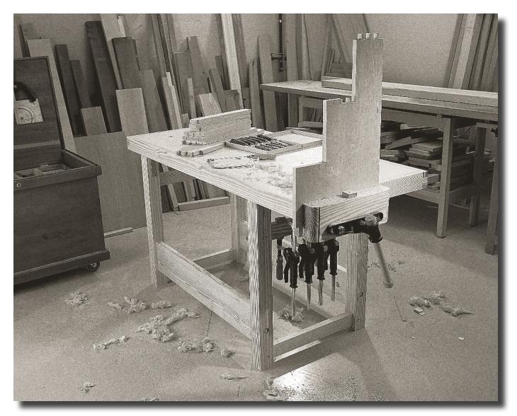
**BUILT TO TRAVEL.** This bench can be knocked flat in about 10 minutes with a <sup>3</sup>/<sub>4</sub>" ratchet set and a No. 3 Phillips screwdriver. I traveled all over the country with this workbench and became quite familiar with its assembly and disassembly. Finally, we gave the bench away to a reader of our magazine who won it in a contest. That guy made the moves on my managing editor, and so did the next reader who won one of my workbenches. So we stopped giving them away.
