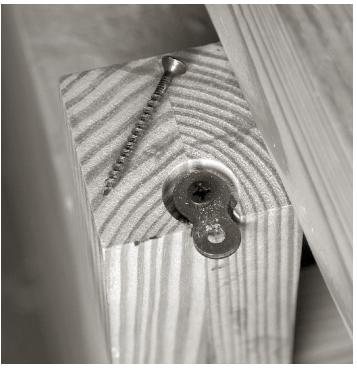
**TOUGH ENOUGH.** Here I attached the top to the base with a figure-8 fastener. The bench's rigidity is maintained by the stretchers below. So the method of attaching the base to the top is more about shear forces than racking forces. So the steel screws do the job quite well.
