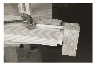
A DOWEL SHOWS THE WAY. Here you can see the jig that indicates where the nut will be located on my stretcher (top). The bottom dowel goes into the bolt hole. The top dowel mirrors the direction of the bottom dowel. The nail pricks the stretcher. That is where your nut will go.
