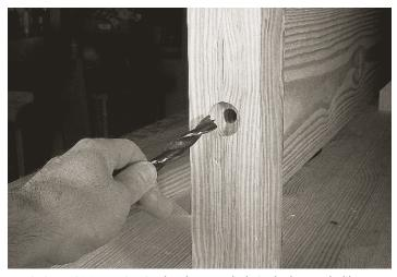
**THIS IS A DOWELING JIG.** The clearance hole in the leg works like a doweling jig to make the clearance hole in the stretcher. The hole in the leg guides the bit as you begin the hole in the stretcher.
