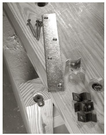
**INEXPENSIVE AND FAST.** You can use hardware designed for attaching dining tables (shown in leg and at right), or beefy steel-plated stuff designed to reinforce garden gates and barn doors.
