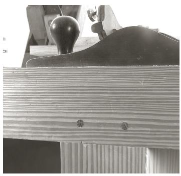
**PERMANENT DRAWBORE.** The base of my French workbench is joined to its top with a large drawbored tenon. It's stout, but makes moving the bench difficult.
