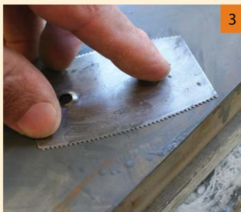
**3 Flatten the back of the blade.** On the same stone, flatten the back of the saw blade. You may want to advance to finer grit stones for a more polished blade. I find a smoother blade is easier to keep clean and rust-free.
