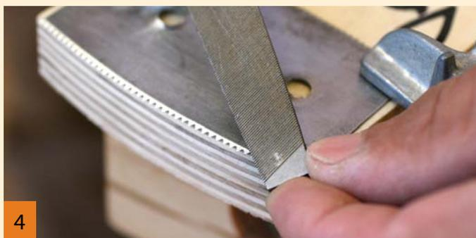
**4 Bevel the cutting edge.** I use a 6” mill file to bevel the cutting edge on one side. Holding the file at an angle and working across the teeth, gently file until a bevel extends from the points to the gullets of the teeth. This (step) produces slender teeth that glide through veneer.
