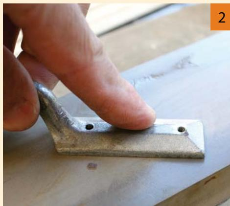
**2 Flatten the spine.** Any bumps or unevenness of the spine against the blade may result in a curved blade that won’t easily cut to a straight line. To establish a flat spine, flatten the back of the spine where it attaches to the blade on a coarse sharpening stone.
