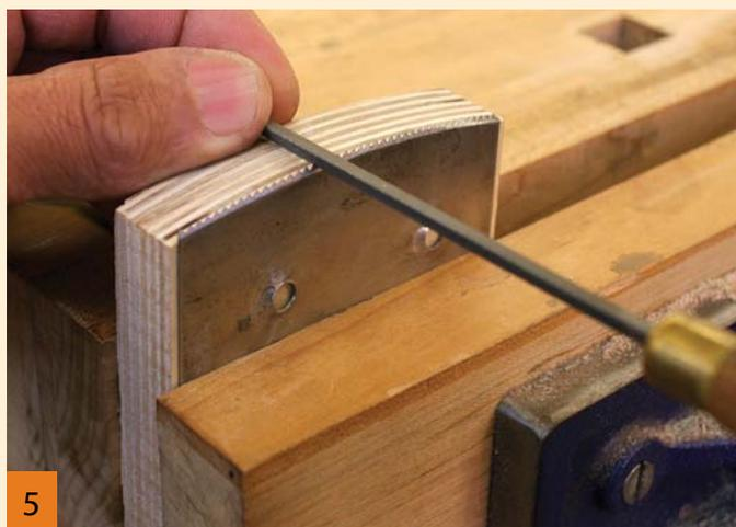
**5 File the teeth.** Using a 4” double extra-slim tapered saw file, I gently bring each tooth up to a nice point. I keep the file at 90° to the teeth and file it just like a rip saw. The exact angle of the teeth isn’t as important as their sharpness, so if your first effort isn’t perfect, don’t worry.
