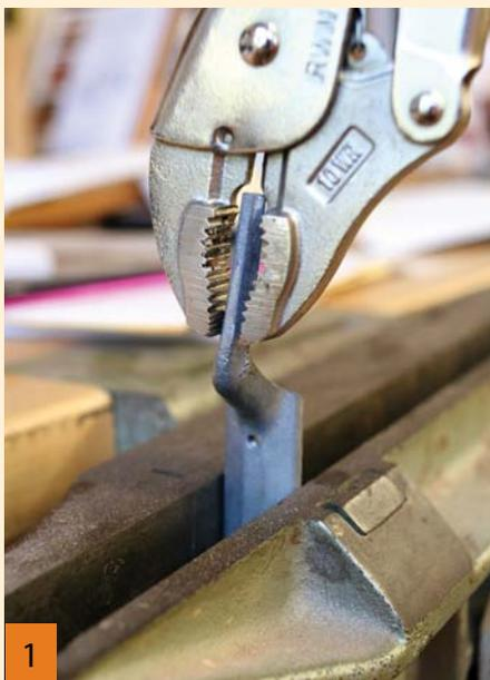
**1 Straighten the tang.** Most veneer saws have an uncomfortable hang (the angle of the handle to the blade). I found that by lowering the handle and placing it more in line with the saw blade, I got better control and improved results with less pressure.
