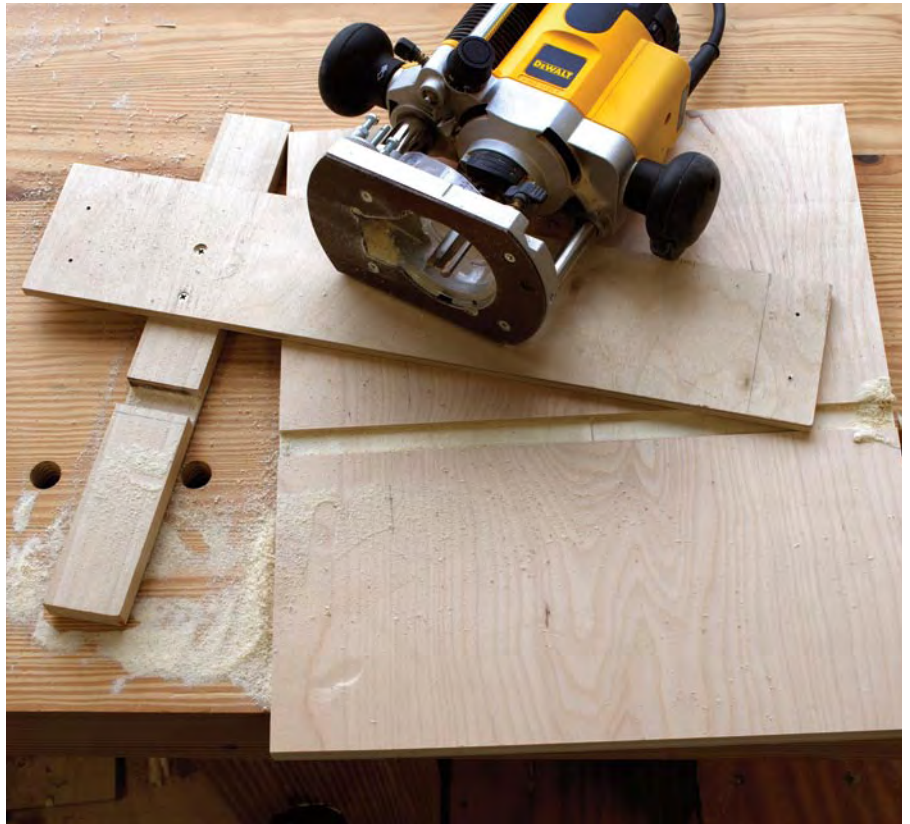
In the groove. Maneuvering a large piece of wood across a stationary machine can be inefficient and yield less-than-perfect results. Take the easy way out and cut dados with a router and this simple jig.
