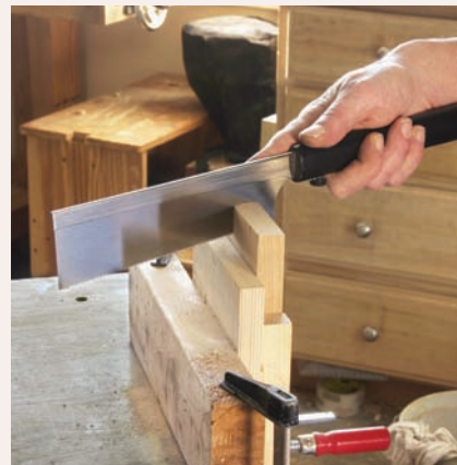
A good start. Many woodworkers start with a Japanese Dozuki as their first joinery saw. It is sharp, functional and doesn't cost a fortune.
