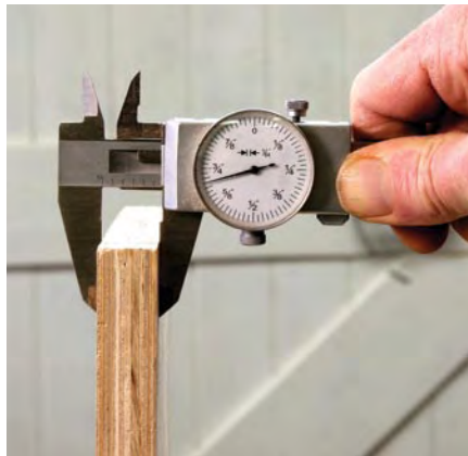
Time to be picky. Dial calipers will quickly give an accurate measurement. Knowing the size you need is key to obtaining a good fit.
