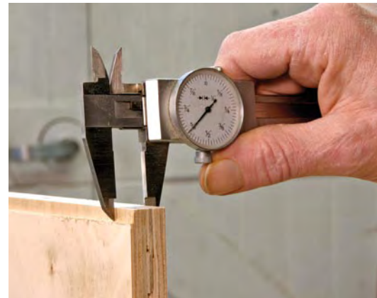
The fix for plywood. Most plywood varies so much in thickness that a good match isn't possible. A small rabbet makes a good joint manageable.
