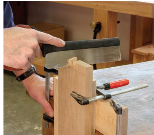
Three clamps and you're ready. With the work clamped to the jig, and the jig clamped to your bench, you can practice making cuts with a handsaw.
