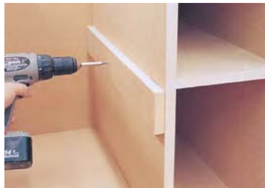
STEP 8 Install the two shelf supports F in the middle section. They are secured with glue and 1\frac{1}{4} " screws. Their top edges are 12\frac{3}{4} " above the bottom board. Cut the middle shelf G to the size indicated in the materials list and secure it to the cleats with glue and brad nails.
