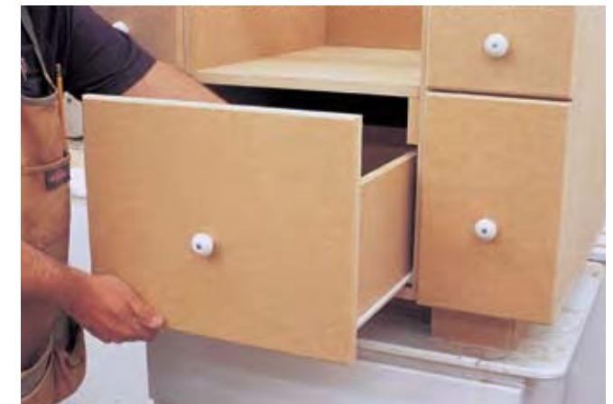
STEP 14 Round over the front edges of drawer face W using a \frac{1}{4} " router bit. Attach it to the drawer box with 1\frac{1}{4} " screws, being careful to leave equal spacing on both sides, with its top aligned to the two outside drawer faces.
