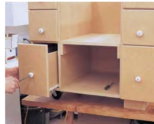
STEP 10 Cut and attach the four stop cleats N with glue and 1\frac{1}{4} "-long screws. These cleats will stop the slide-out when fully extended. When it's necessary to remove or install the slide-outs, simply tip them upward to move past the stop cleats.
