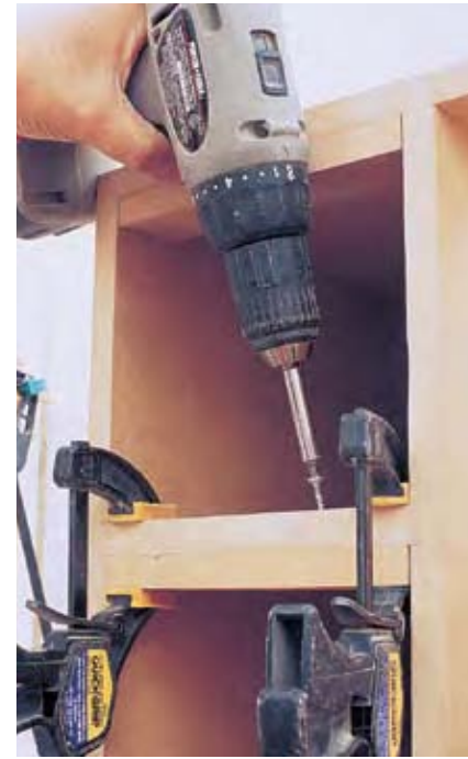
STEP 10 Cut and attach the four stop cleats N with glue and 1\frac{1}{4} "-long screws. These cleats will stop the slide-out when fully extended. When it's necessary to remove or install the slide-outs, simply tip them upward to move past the stop cleats.
