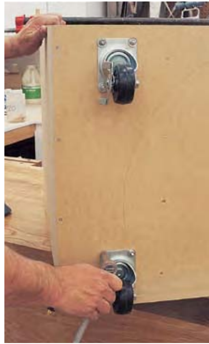
STEP 6 If you plan to use base option #1, attach two heavy-duty locking wheel assemblies to one side of the cabinet.
