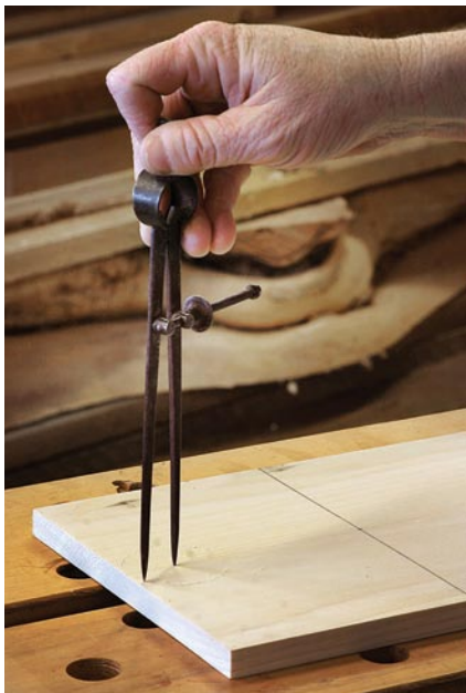
Perfect circles. If you can't find a compass, dividers work just fine for marking out circles – and the resulting tool marks add an air of period flair.
