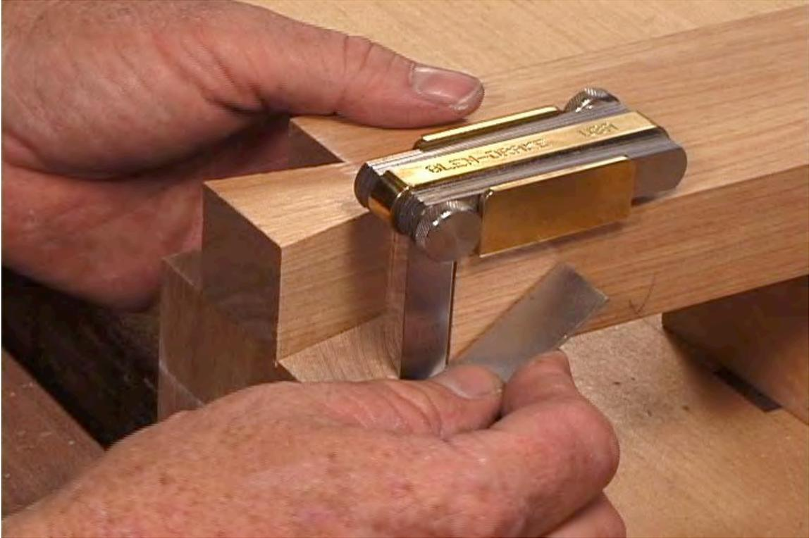
12. Use your Kerf-Starter along the left side of the tail to mark the left side of the tail socket.
