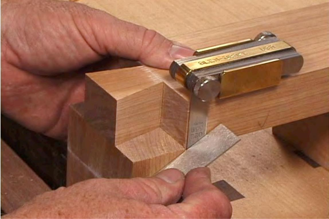
9. Use the blade of your square to flush-up the tail edge with the pin edge, using the offset blade as a spacer. This will shift the tail piece to the left.
