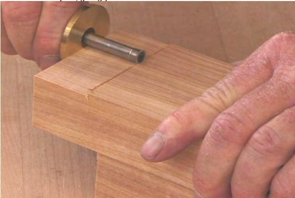
2. Use your Tite-Mark to pare the rabbit down to the shoulder line and then carry that line all the way around the tail piece to establish a shoulder line that lines up precisely with the shoulder of the rabbit.
