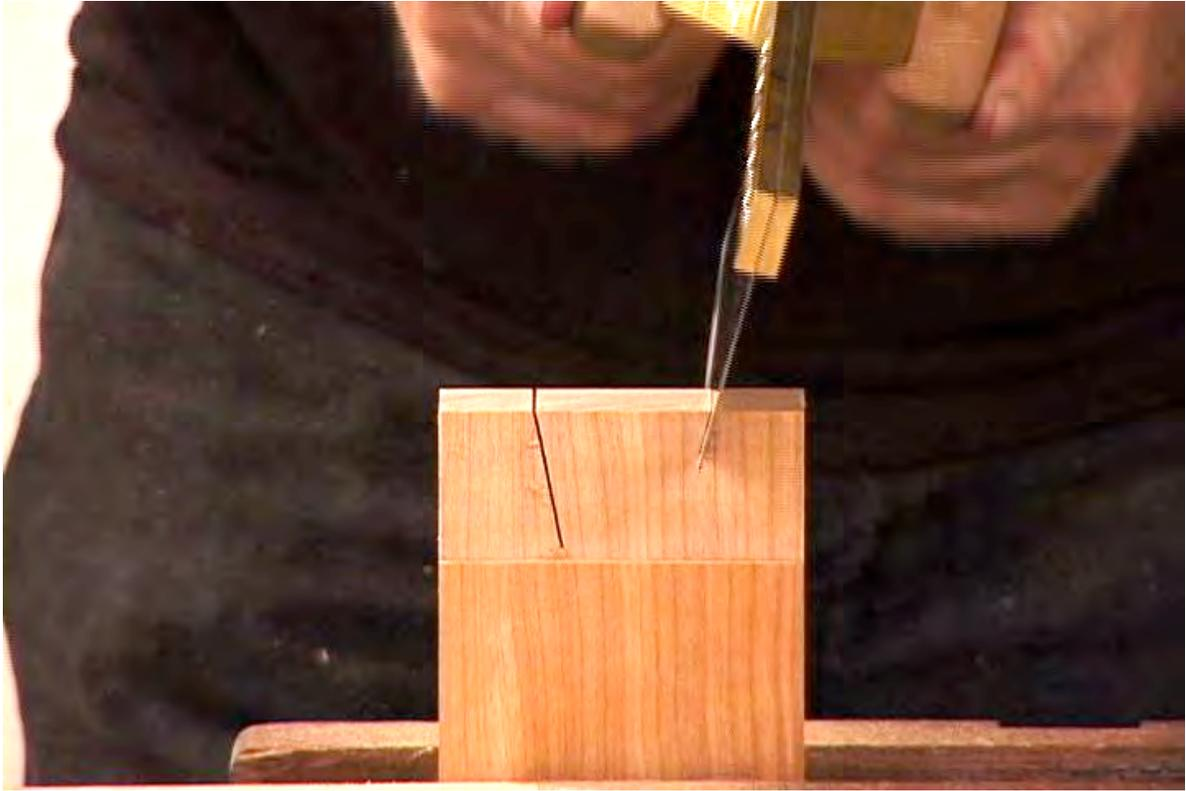
4. Remove the waste by sawing above the shoulder and then chop down to the shoulder line to make the shoulders nice and crisp.
