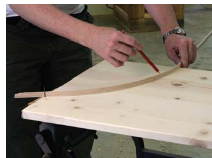
Mark a curve. A nail acts as a third hand while I mark the concave curve at the top of one side piece.
