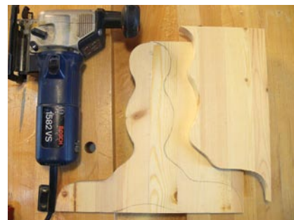
Pattern. Use the offcut from the first half of your side piece to mark the matching shape on the remaining three cuts.
