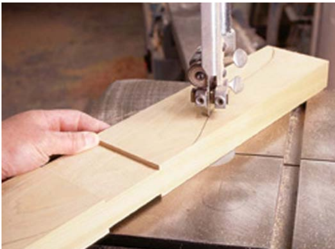
Sculpting a shape on the cross braces isn't necessary to keep the table sturdy, but it does keep it from looking clunky. After transferring the pattern onto the brace, I cut wide of the line on the band saw, then used a spindle sander to smooth the shape.
