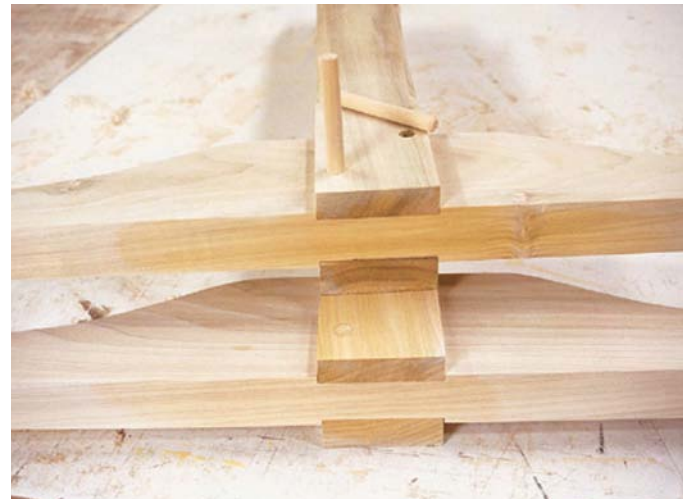
With the cross braces glued to the posts, they are pegged in position. Clamp them tight and check for square between the post and brace. Note that the pegs are at opposite corners of the joint. This allows room for the mortise (in the next step).
