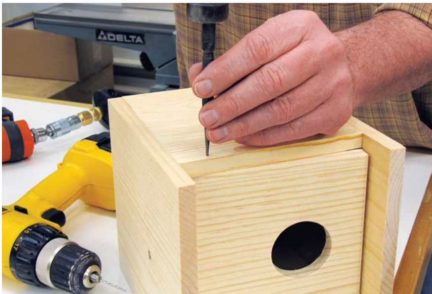
FIGURE 3 Use a nail set to put the heads of the hinge nails slightly below the surface.
