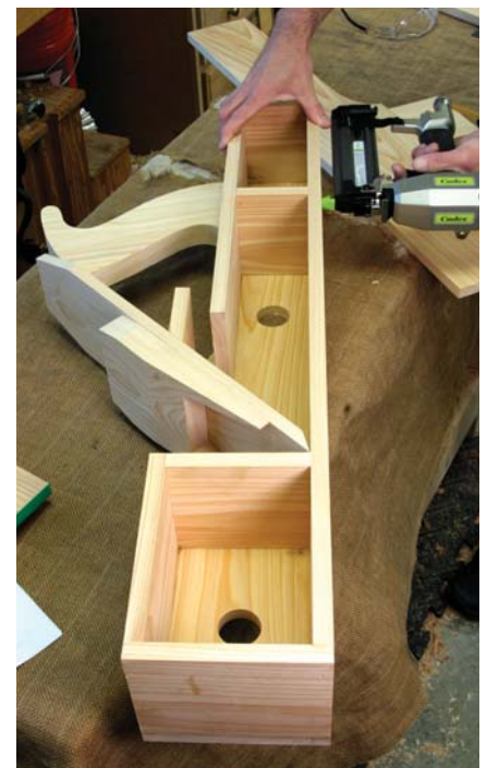
THIS PLANE IS HOLLOW. Glue and nail all the interior pieces as shown before you screw the second sidewall in place.
