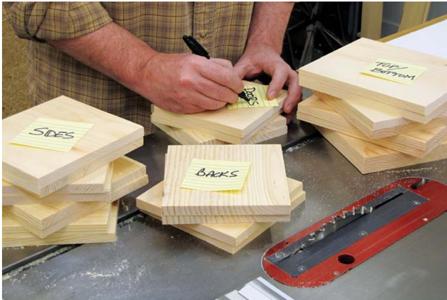
FIGURE 1 With the exception of the top/bottom components, which are identical, all the house parts are very similar in size, so label your stacks to keep everything straight.
