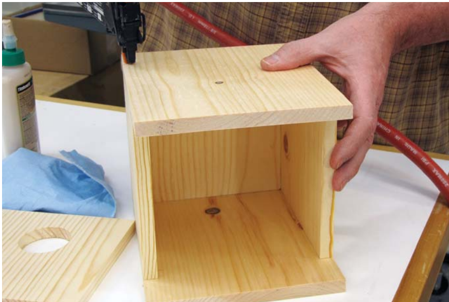
FIGURE 2 With waterproof glue and nails, begin the assembly by attaching the house sides to the house back. To this assembly, attach the top and bottom pieces.
