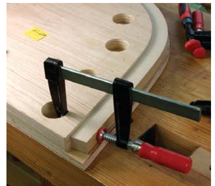
Flexible terms. Compwood can be bent without steam or—in many cases—a bending strap. It also can be bent in three dimensions.
