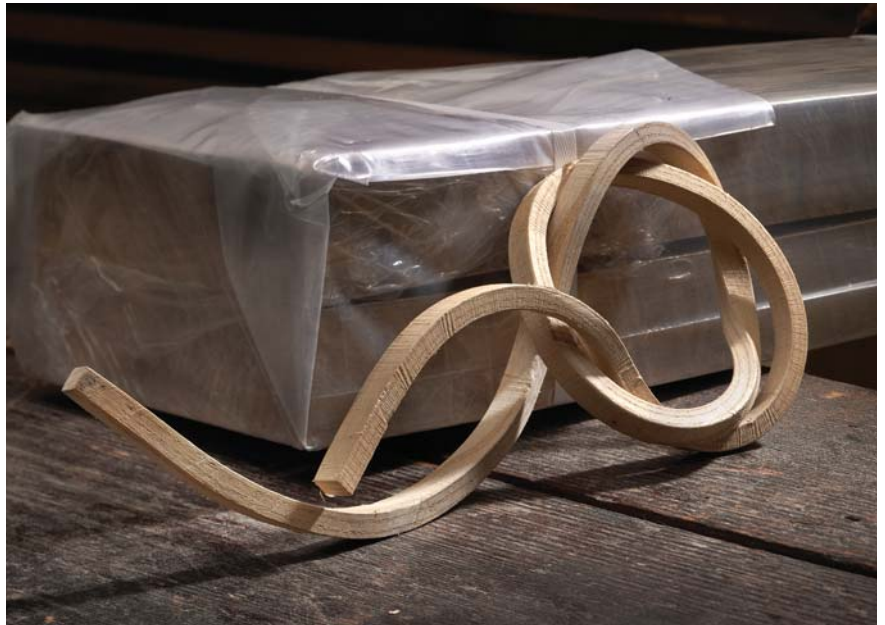
I can bend that. With Compwood, you can bend wood in ways that are surprising. When the wood dries, it holds its shape and can be worked with standard woodworking tools.
