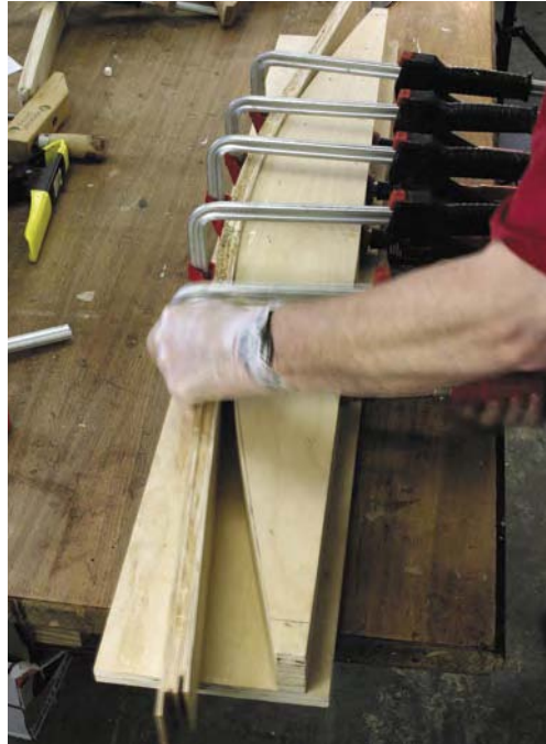
Starting at the center and working out to each end, clamps are placed every 4" to 5" around the form.
