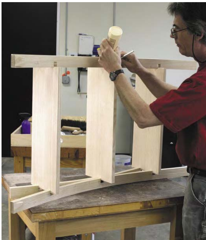
Line up the shelves in the notches, then brush glue on all surfaces of the joint.
