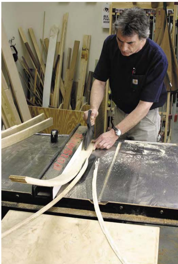
The other edge is ripped on the table saw, maintaining contact with the table on the infeed side of the saw blade.
