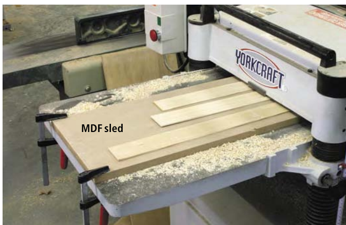
Thin pieces can be sent through the planer on a sled, a piece of \frac{3}{4} "-thick MDF that extends past the feed rollers and is clamped to the planer bed.
