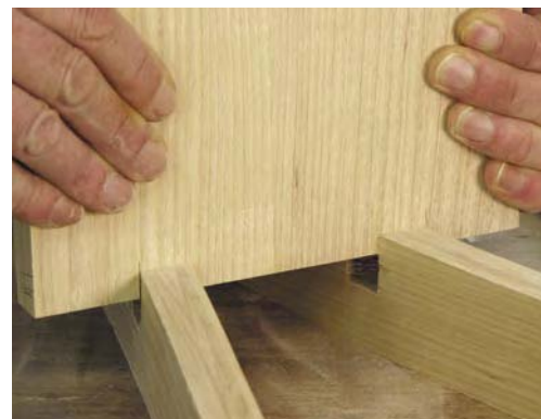
The ends of the shelves fit in the notches. Adjust the fit with a few swipes with a smoothing plane. Mark the support locations on the bottom of the shelves to keep the parts in line during assembly.
