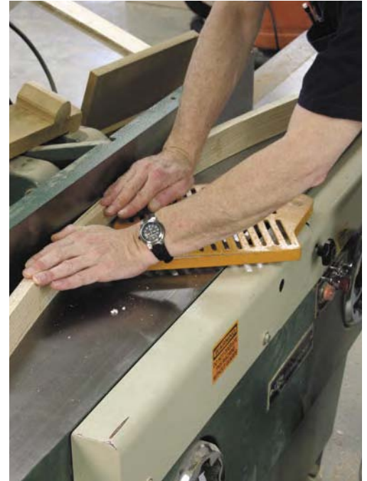
After scraping off the excess glue, one edge is evened up on the jointer. Make sure to keep the curve in contact with the fence on the outfeed side of the cutterhead.
