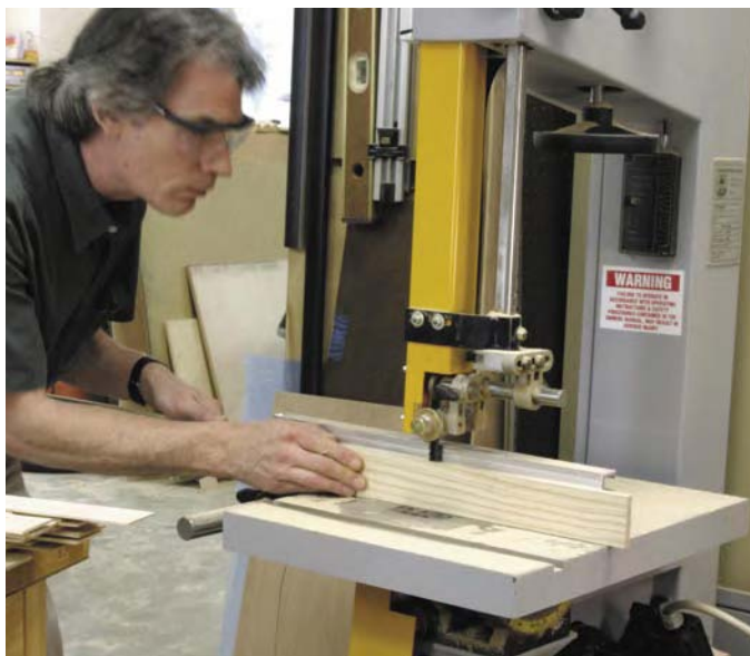
Resawing strips on the band saw is safer and less wasteful than using the table saw. I cut them a little thicker than necessary, clean up the saw marks, and bring them to final thickness with the planer.
