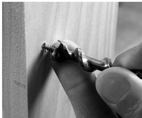
The pilot hole helps guide all subsequent boring operations. For the counterbore, place the lead screw in the pilot hole.
