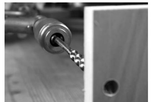
When the lead screw poked through the exit side of this hole I stopped turning the handle, removed the auger and began the cut on the exit side. This eliminates the grain from blowing out as the bit clears your work.
